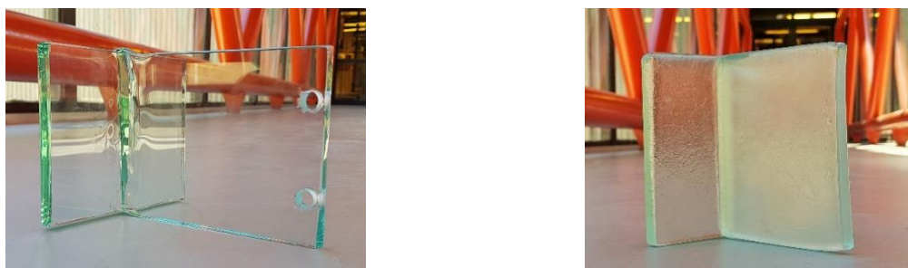
Fig. 1 Welded T-section (left) and fused T-section (right).
