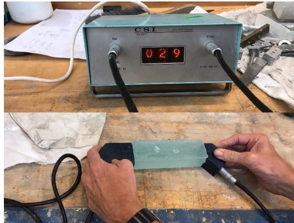
Fig. 11 The ultrasonic method for Young's modulus testing, photo by author.
