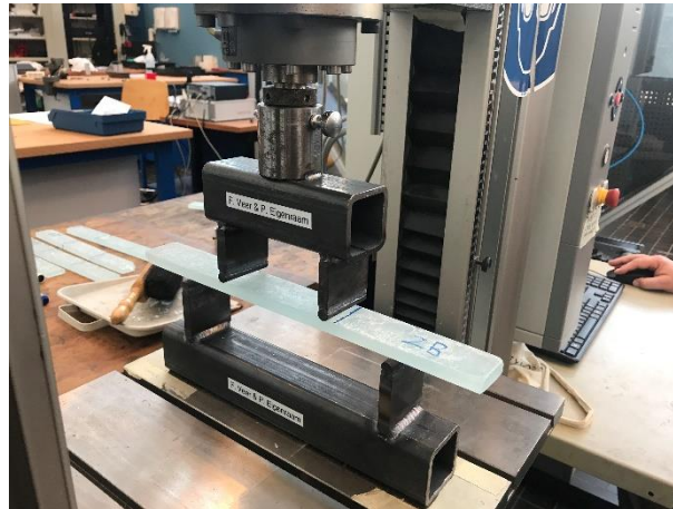
Fig. 15 The four-point bending test for sample 5 to 10, photo by author.
