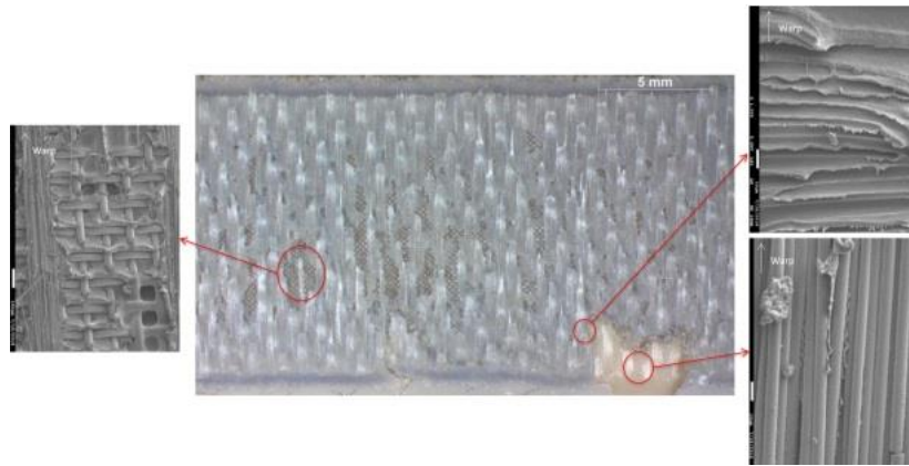
Figure 2.14. Fracture surface of specimen tested at 120 °C (centre). SEM micrographs illustrate the fibre/matrix debonding (right) and mesh/matrix debonding (left). The top right SEM image illustrates fibre imprints in the resin and the bottom right SEM image illustrates debonded fibres.
