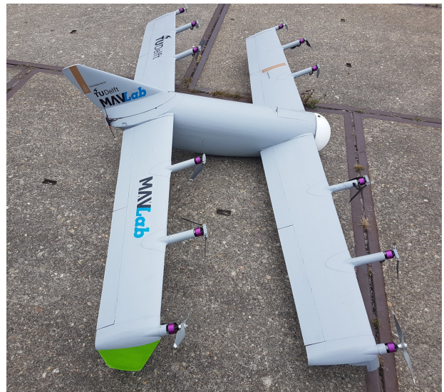
Fig. 1. NederDrone2 with 12 propellers of which 8 are foldable and stop during forward flight. The 4 tip propellers remain active during forward flight and have a higher pitch for efficient fast flight. The large fuselage can accommodate a 9 liter pressure tank and a fuel-cell.
