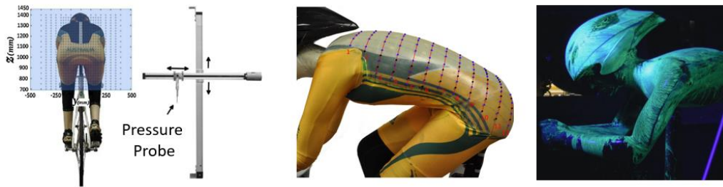
Figure 1.6: Measurement techniques adopted for cycling aerodynamic research: pressure probe scanning the wake (left; adopted from Crouch 2013); pressure taps on the cyclist's back (middle; adopted from Crouch et al. 2014); China clay visualization depicting separation line on upper arm (right; adopted from Brownlie et al. 2009).
