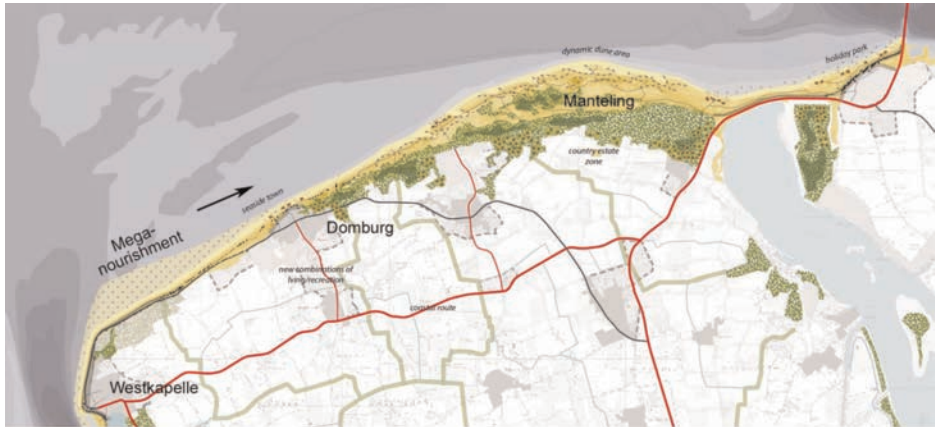
Figure 6: Mega-nourishment design for west-Walcheren feeding the waterfront of Domburg, with dynamic dunes for the ecology of the Manteling (Studio Coastal Quality, TUD)
