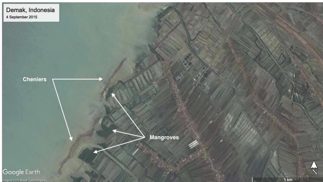
Figure 2. Google Earth image [17] taken on 4 September 2015 shows two cheniers off the coastline of Demak. Behind those cheniers, some small patches of mangrove forest are visible. North of the cheniers, where the coastline is unprotected, barely any mangrove tree persists.
