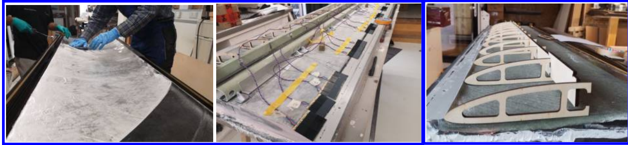
(a) Laminating top skin. (b) Spars and wing components alignment. (c) Rib assembly.
