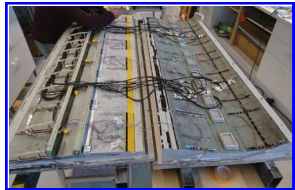
(b) Integrating smart sensors, actuators and components in the wing.
