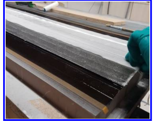
(b) Process of ply dropping fibre glass layers.
