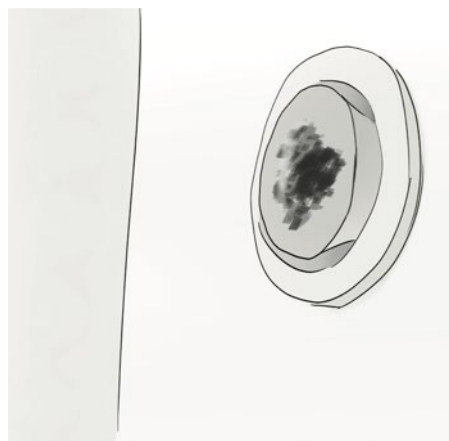
Figure 17 Indicating the need to clean valves right at the place of the valve itself.
