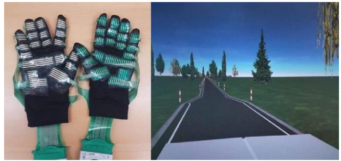
Figure 2. The used grip force sensors (left), and the simulator environment (right) for the 500m road narrowing including the car front.
