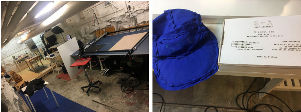
Figure 4 Small self-assembly studio with self-built open-source laser cutter (left) and an S-A cap showing the special seams. The mailing package has laser-engraved instructions (right). Source: Natalia Särmäkari.
