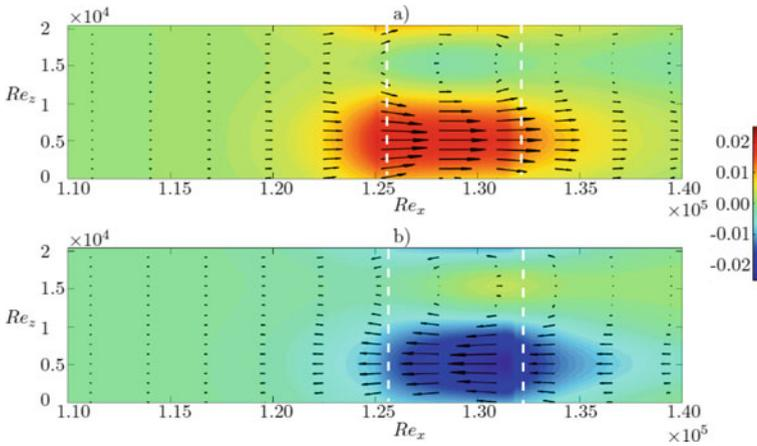
**Fig. 24** Induced streamwise velocity vectors superimposed onto the induced stream for **a** co-flow (case 2) and **b** wise velocity contours on an x-z plane at  $y = 0.1 \delta_{1,0}$  counter-flow (case 4) actuations with straight-edged electrodes. The DBD position and shape is indicated by the white dashed lines
