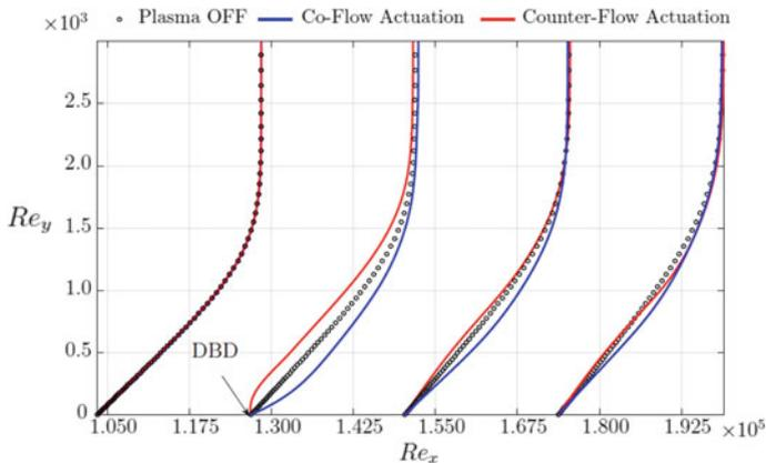
**Fig. 22** Streamwise velocity profiles for no-actuation (black circles), co-flow (blue solid line, case 2) and counter-flow (red solid line, case 4) actuations with straight-edged electrodes. The DBD actuator location is indicated by an arrow
