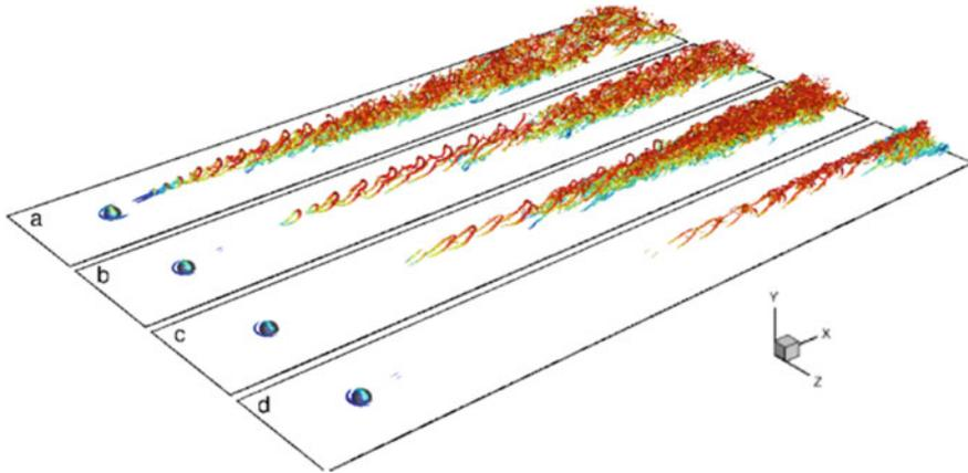
**Fig. 39** Coherent vertical structures for flow around hemispherical roughness element. **a**  $M_\infty = 1.1$ ,  $Re_\delta = 6500$ ; **b**  $M_\infty = 2$ ,  $Re_\delta = 9000$ ; **c**  $M_\infty = 4$ ,  $Re_\delta = 40000$ ; **d**  $M_\infty = 6$ ,  $Re_\delta = 85000$ . Vortices are educed as isosurfaces of swirling strength, and coloured with the streamwise velocity
