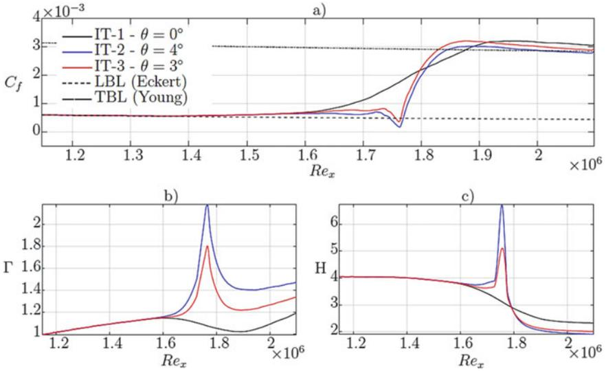
**Fig. 72** Time- and span-averaged skin friction (a), displacement thickness (b) and shape factor (c) distributions for  $\theta = 4^\circ$  (blue solid line),  $\theta = 3^\circ$  (red solid line) and ZPG (black solid line—case IT-1). Laminar (dashed-dotted black) and turbulent (dashed black) boundary-layer distributions by [9] and [10], respectively
