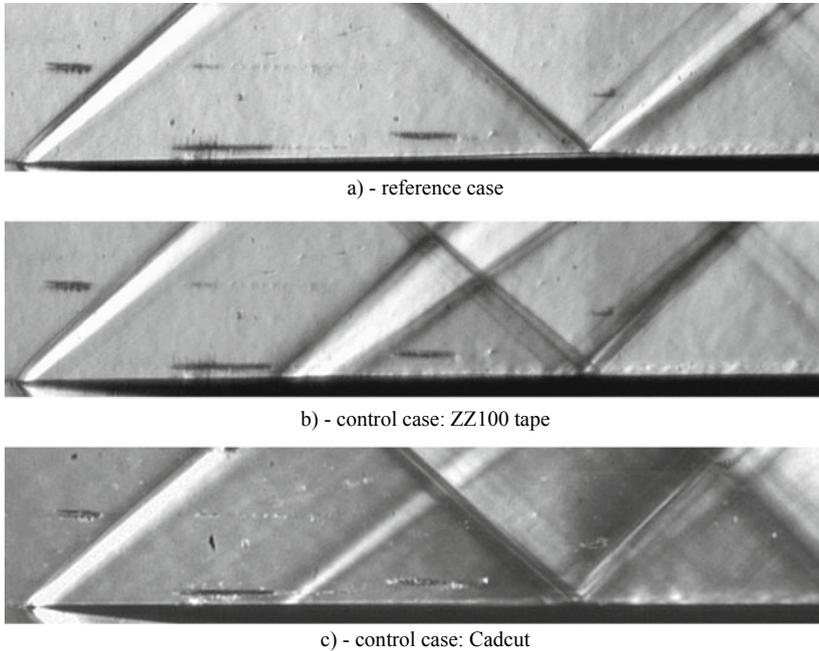
**Fig. 57** Schlieren visualizations (devices at  $X_{d1}$  location)
