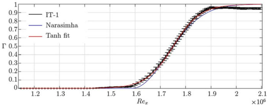
**Fig. 71** DNS span averaged intermittency distribution (black solid line with error bars due to the threshold sensitivity) for the ZPG boundary-layer at  $Re_{\delta_{1,0}} = 2835.84$  (case IT-1). Narasimha (blue solid line) and hyperbolic tangent (red solid line) fit curves are also plotted
