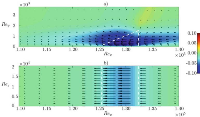
**Fig. 25** Induced streamwise velocity vectors superimposed onto the induced streamwise velocity contours on **a** a x-y plane at  $z = L_z/4$  and **b** a x-z plane at  $y = 0.1 \delta_{1,0}$  for counter-flow actuation with straight-edged electrodes and no electric field spanwise variation (case 5). The DBD position and shape is indicated by the white dashed lines
