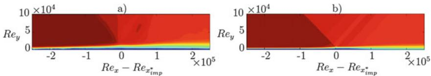
**Fig. 74** Contours of instantaneous streamwise velocity from PIV measurements by ITAM (a) and LES-MTS (b). Levels between 0.0–1.0. (With permission of A. A. Sidorenko and P. A. Polivanov at the Institute of Theoretical and Applied Mechanics from Novosibirsk State University)
