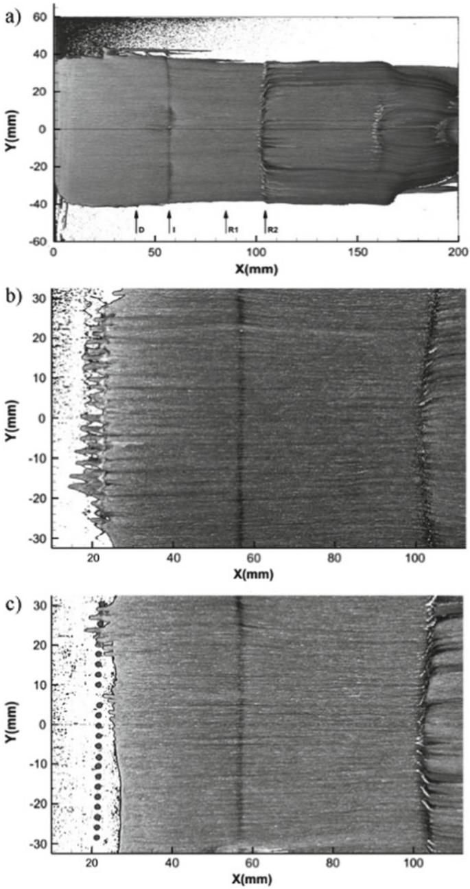
Fig. 58 Oil flow visualizations (devices at  $X_{d1}$  location)
