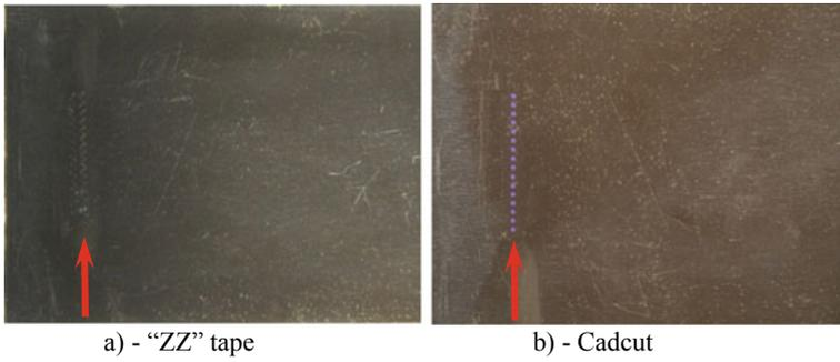
Fig. 14 Turbulator devices mounted on the flat plate
