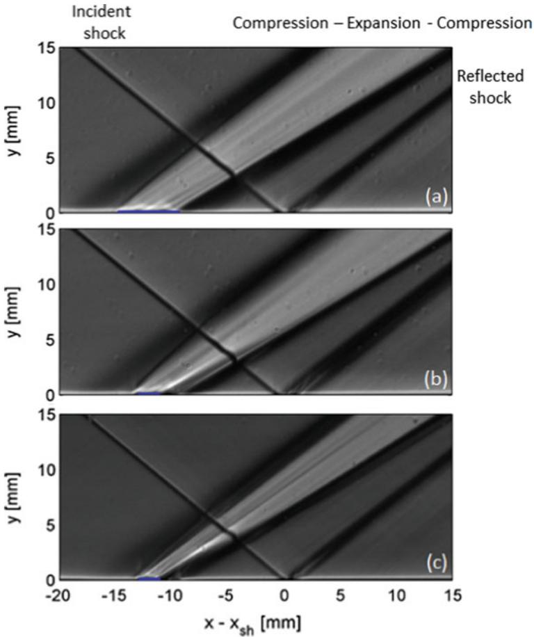
**Fig. 65** Schlieren visualizations of the interaction for three tripping devices positioned 10 mm upstream of an impinging oblique shock wave ( $x_{sh} = 51$  mm). **a** zig-zag strip; **b** step; **c** distributed roughness
