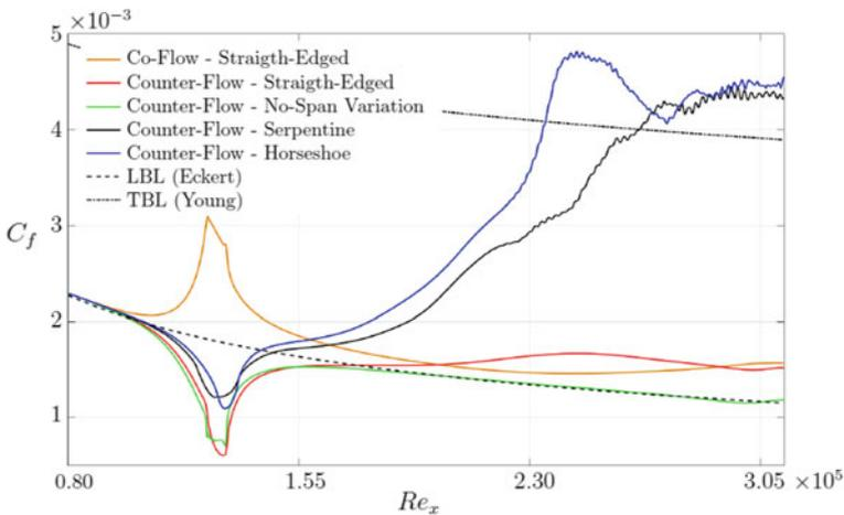
**Fig. 28** Time and span-averaged skin friction distributions for different plasma actuation configurations. Cases: 2 (orange solid line), 4 (red solid line), 5 (green solid line), 6 (black solid line) and 9 (blue solid line). Laminar (black dashed line) [9] and turbulent (black chain-dotted line) [10] boundary-layer distributions are also plotted
