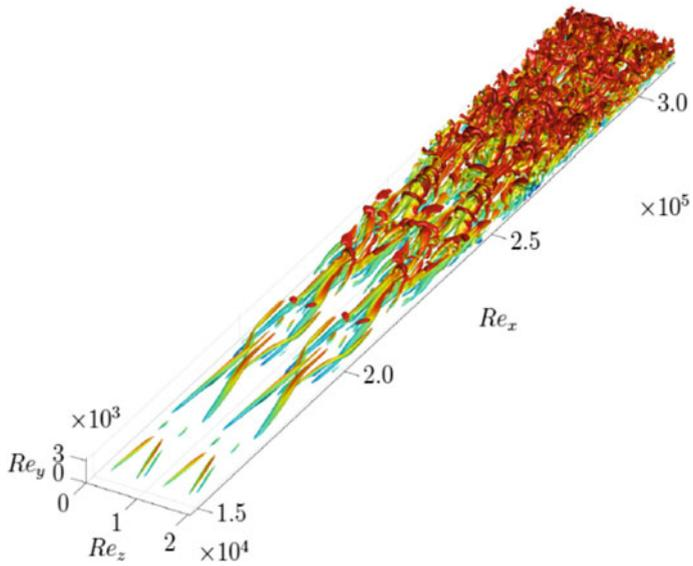
**Fig. 33** Iso-surfaces of Q-criterion for horseshoe counter-flow actuation
