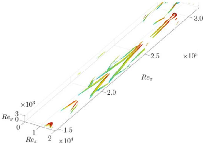
**Fig. 31** Iso-surfaces of Q-criterion for straight-edged counter-flow actuation
