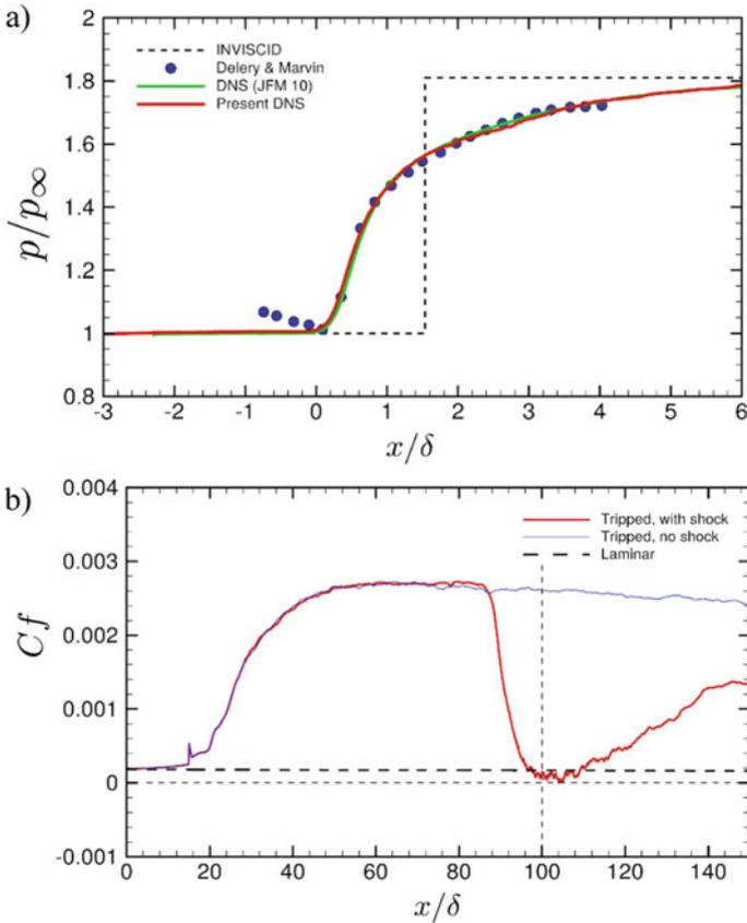
**Fig. 47** Distribution of mean wall pressure (a) and skin friction coefficient (b). *R-H* denotes the inviscid distribution resulting from the Rankine-Hugoniot jump conditions. Refer to Table 7 for nomenclature of symbols
