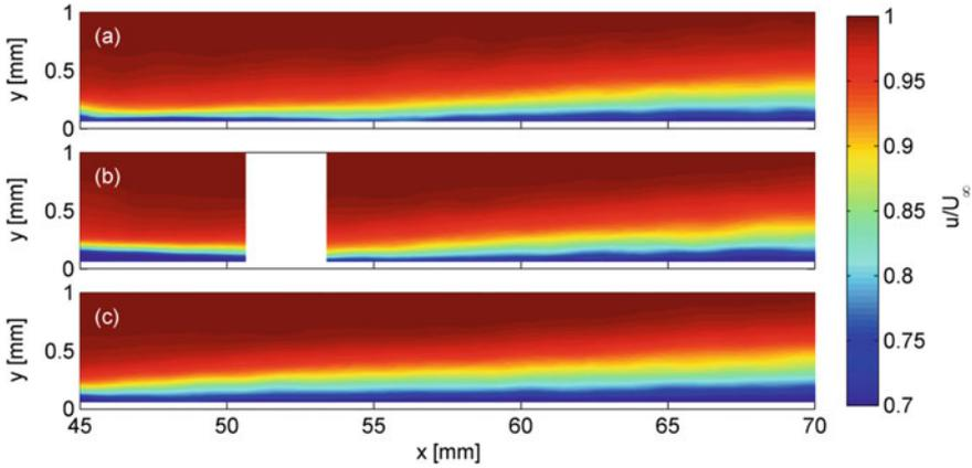
**Fig. 16** Streamwise component of the velocity field downstream of the transition control devices. **a** zig-zag strip **b** step **c** distributed roughness patch
