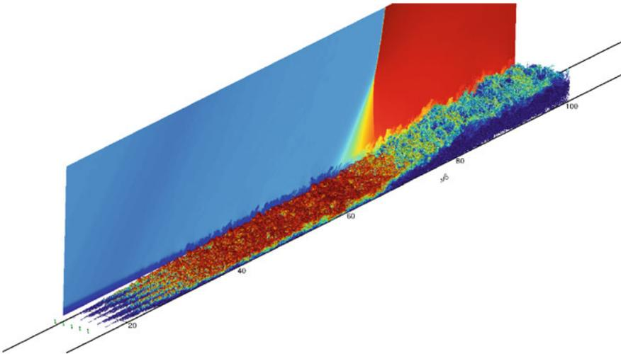
**Fig. 49** Flow visualization for turbulent interaction at  $M_s = 1.3$ . Vortical structures are educed through iso-surfaces of the swirling strength. The pressure field is also shown in a  $x$ - $y$  plane slice
