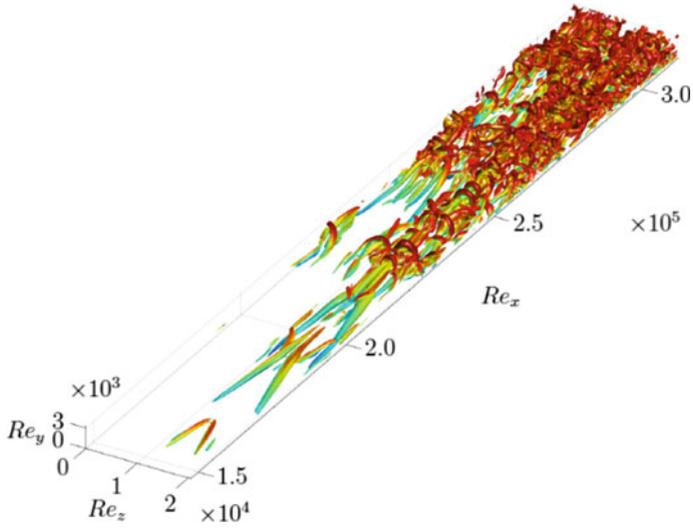
**Fig. 32** Iso-surfaces of Q-criterion for serpentine counter-flow actuation
