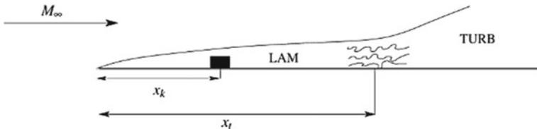
**Fig. 34** Sketch of boundary layer transition induced by an isolated roughness element.  $M_\infty$  is the Mach number of the (compressible) boundary layer,  $x_k$  is the distance of the roughness element by the plate leading edge and  $x_t$  indicates the transition location
