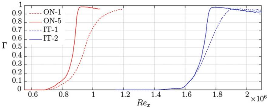
**Fig. 76** Span averaged intermittency distributions for the ZPG (red dashed line—case ON-1) and  $\theta = 4^\circ$  (red solid line—case ON-5) cases at  $Re_{\delta_{1,0}} = 1971.07$  and the ZPG (blue dashed line—case IT-1) and  $\theta = 4^\circ$  (blue solid line—case IT-2) cases at  $Re_{\delta_{1,0}} = 2835.84$
