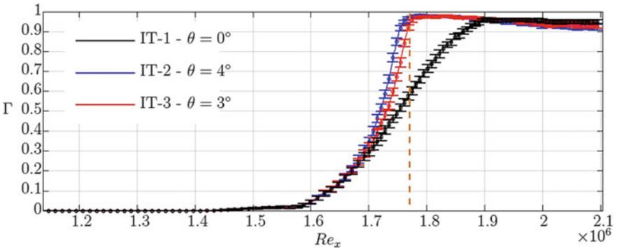
**Fig. 73** Span averaged intermittency distributions (with error bars due to the threshold sensitivity) for the transitional case with  $\theta = 4^\circ$  (blue solid line—case IT-2) and  $\theta = 3^\circ$  (red solid line—case IT-3). The ZPG boundary-layer (black solid line—case IT-1) is also plotted. The vertical orange dashed line indicates the shock impingement location
