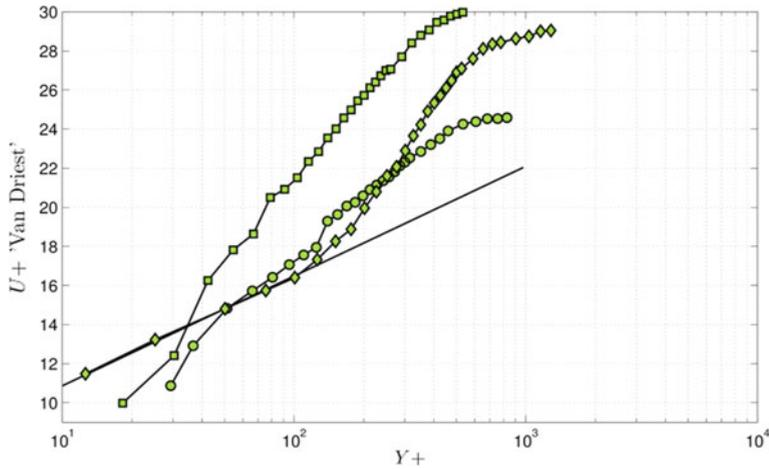
**Fig. 1** Van Driest representation of the velocity profile downstream of the interaction ( $X^* = 0.35$ ),  $\Theta_3$  angle:  $\circ$ : B0,  $P_0 = 0.4$  atm,  $\square$ : B2,  $P_0 = 0.4$  atm,  $\diamond$ : B2,  $P_0 = 0.8$  atm
