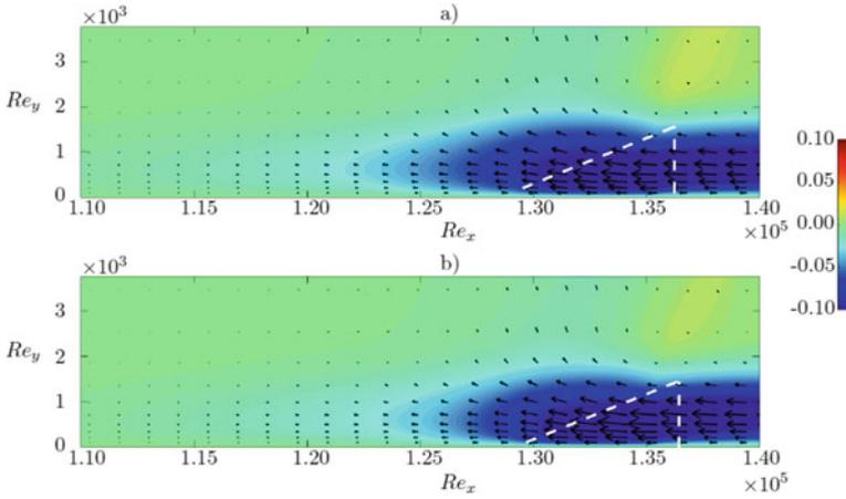
**Fig. 26** Induced streamwise velocity vectors superimposed onto the induced stream-wise velocity contours on an  $x$ - $y$  plane at  $z = L_z/4$  for counter-flow actuation with **a** serpentine (case 6) and **b** horseshoe (case 9) electrodes. The DBD position and shape is indicated by the white dashed lines
