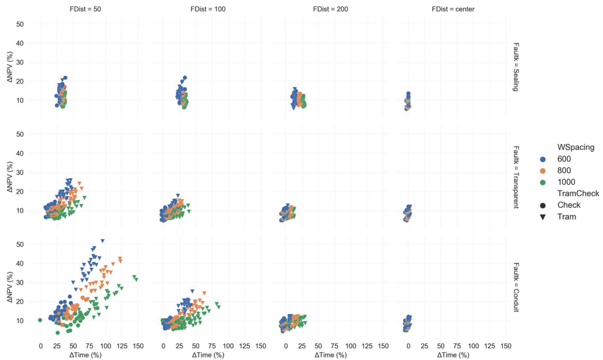
Fig. 19. Changes in system lifetime and NPV between a single developer (mean) (0,0) and a single developer (separate) for a flow rate of 400 m 3 /h.
