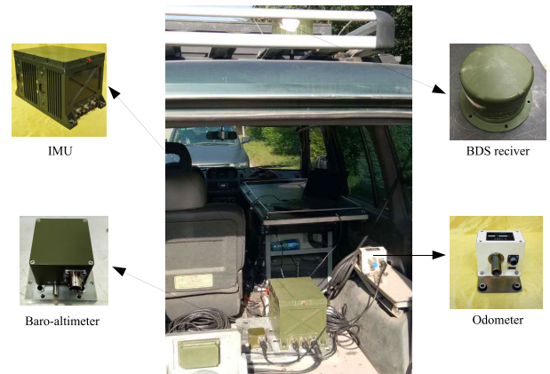
FIGURE 5. Hardware structure of the ground vehicle navigation system.
