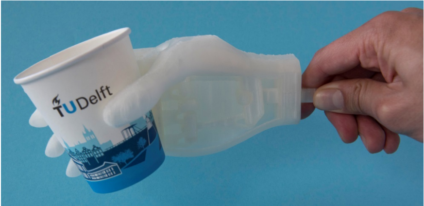
Figure 9.1: The non-assembly prosthetic hand described in Chapter 4 of this thesis.
