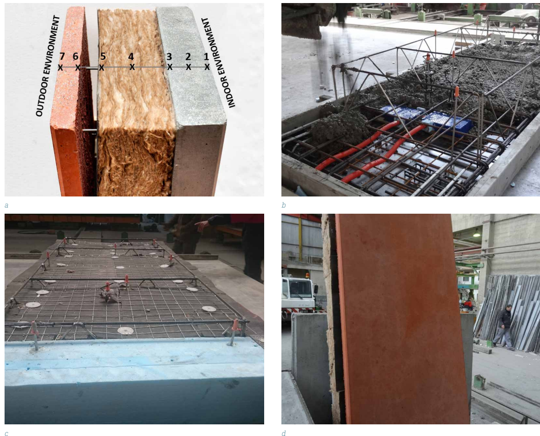
FIG. 3 Prefabricated RAC façade panel: a) model; b)-d) production phases in precast factory
