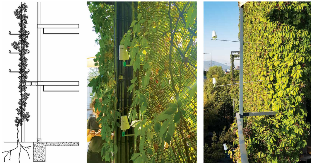
FIG. 1 Schematic section and north-west façade of Case 1
