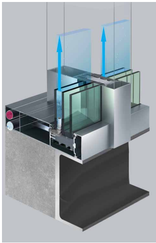
FIG. 1 Typical layout of Water House building envelope
