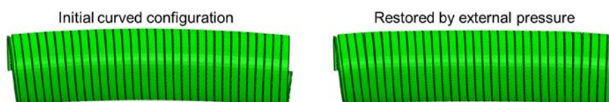
Figure 10. Curved riser (three layers) restored by external pressure to a straight configuration. (This figure is available in colour online.)
