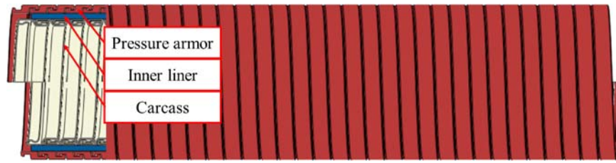
Figure 4. Model-A for investigating the wet collapse mechanism of curved flexible risers. (This figure is available in colour online.)
