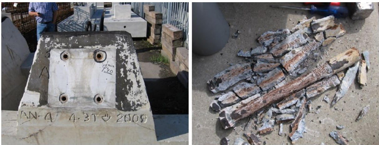
Figure 2.7: Damaged block due to the corrosion of anchor induced by stray current [105].
