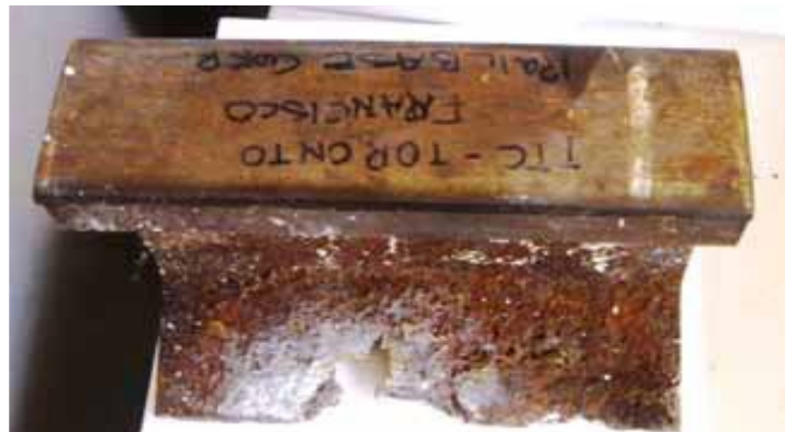
Figure 2.4: View of a section of 115-lb rail showing severe corrosion at the base of the rail [88].
