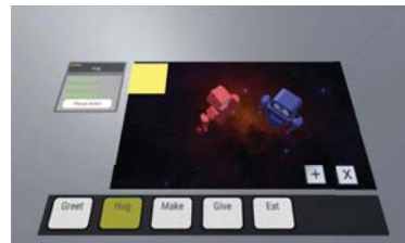
Fig. 2. Marker programming space with marker placed on top of it. The menu appears next to the marker, to choose which content to add.
