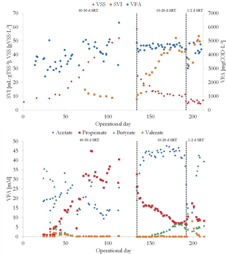
**Figure 2.3** – Upper picture is an overview of the reactor performance in terms of VFA, VSS production and the compactness of the culture expressed as SVI<sub>60</sub>. The bottom picture is the evolution of the product spectrum obtained during each enrichment. Day 0-134 is the 40-50 d SRT, day 135-191 is the 10-20 d SRT and finally day 192-215 is the 1-2 d SRT system.
