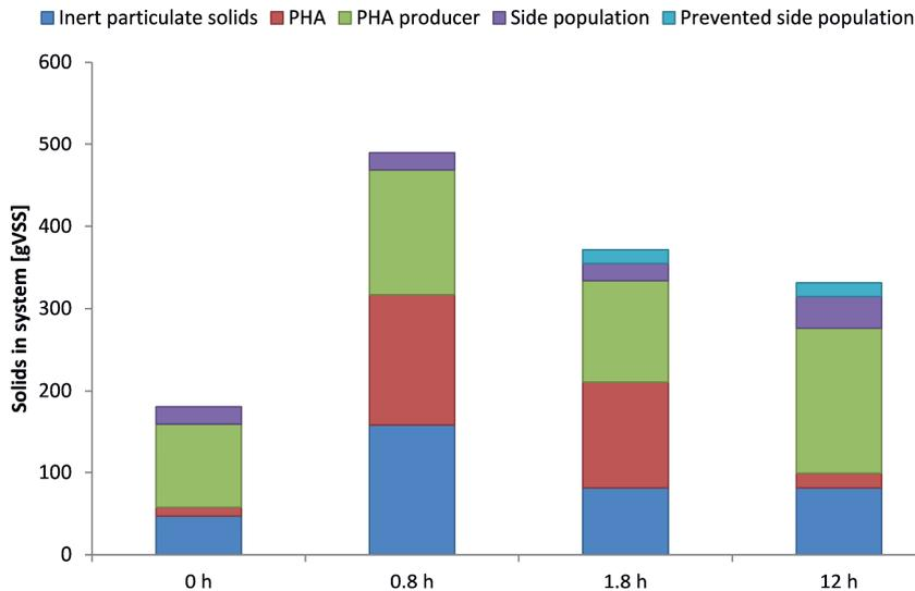
**Figure 5.6 – The solid partition over the cycle. Here 0h represented the beginning of the cycle, 0.8 h represented the time point in the cycle when all VFA were consumed, 1.8 h was the solid composition in the reactor after 1 h settling and removal of the supernatant. Finally, 12 h represents the end of the cycle**
