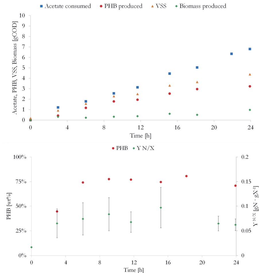
**Figure 4.3 – Nitrogen limited accumulation targeting 80 wt% poly(3-hydroxybutyrate) (PHB) (CODN-26).** The top graph shows the acetate consumed, PHB produced, total amount of volatile suspended solids (VSS) present, biomass produced, all in Chemical Oxygen Demand (COD) equivalents. The bottom graph shows PHB wt% and the yield of NH<sub>4</sub>-N per X produced with a 95% confidence interval.
