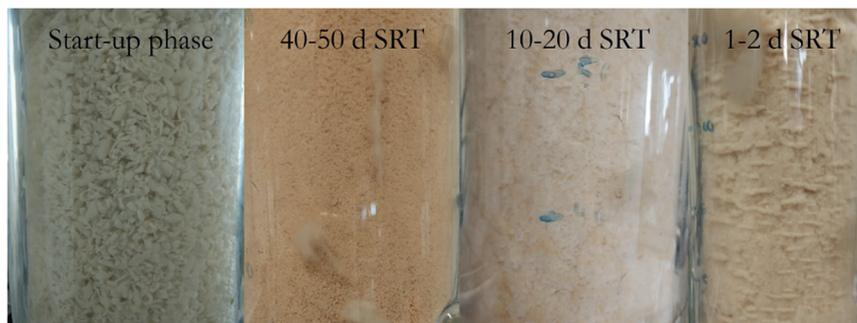
Figure 2.2 – Visual impression of the sludge bed during the different operational periods in this study. From left to right, Start-up phase, 40-50 d SRT, 10-20 d SRT, and 1-2 d SRT.
