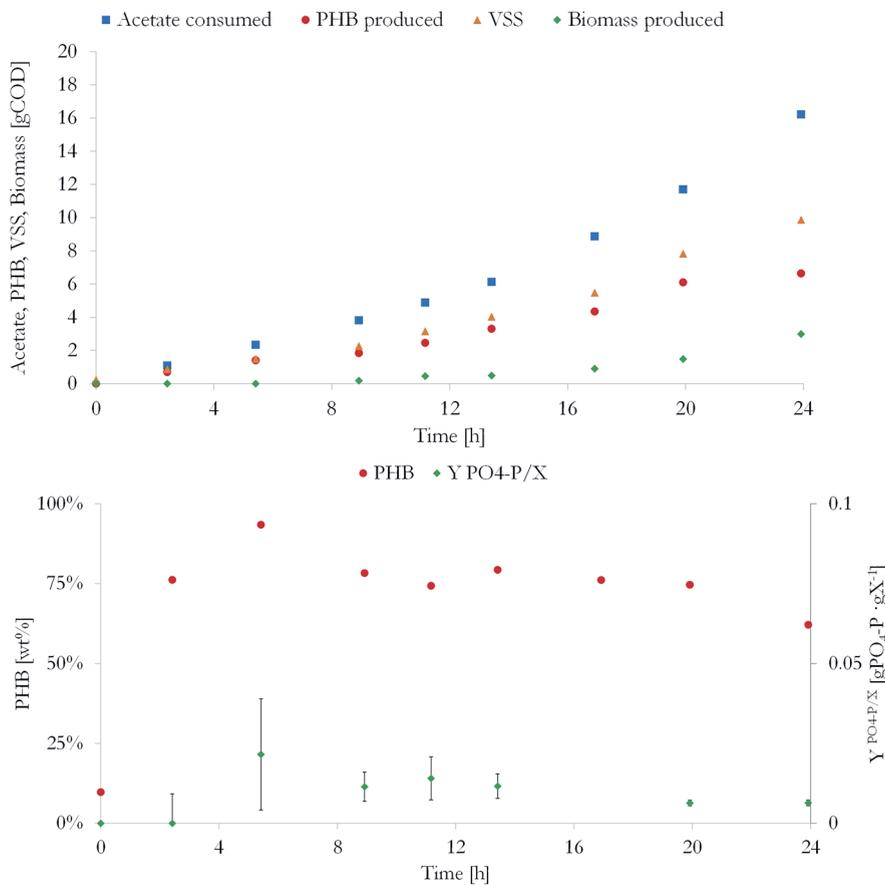
**Figure 4.2 – Phosphorus limited accumulation targeting 80 wt% poly(3-hydroxybutyrate) (PHB) (CODP-511).** The top graph shows the acetate consumed, PHB produced, total amount of volatile suspended solids (VSS) present, biomass produced, all in Chemical Oxygen Demand (COD) equivalents. The bottom graph shows the PHB wt% and the yield of  $\text{PO}_4\text{-P}$  per X produced with a 95% confidence interval.
