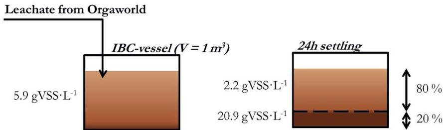
**Figure 6.3.** The effect of the pre-treatment visualized in which untreated leachate was settled for 1 d in a 1 m<sup>3</sup> vessel.
