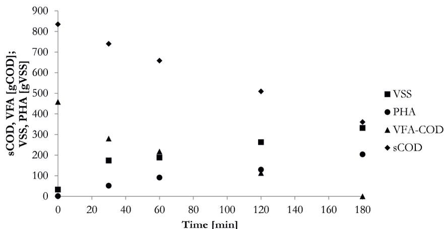
Figure 5.5 – Detailed characterization of a PHA accumulation potential experiment (15-08-2017). Illustrating the evolution of  $\text{COD}_{\text{sol}}$ ,  $\text{COD}_{\text{VFA}}$ , PHA and VSS over time in absolute amounts.
