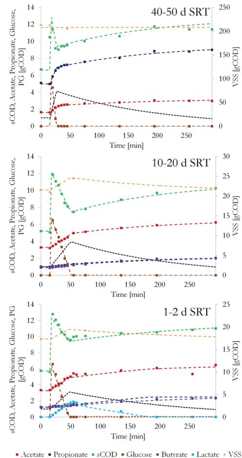
**Figure 2.4** – All system characterisations performed in this study. From top to bottom the 40-50 d SRT, 10-20 d SRT and finally the 1-2 d SRT is depicted. Markers reflect measurements and lines are modelled. Soluble COD concentrations (sCOD) were calculated as the sum of the individual substrate and product concentrations. Cycle measurements were performed at the end of each enrichment thus on days: 134, 191 and 212 for respectively 40-50 d, 10-20 d and 1-2 d SRT.
