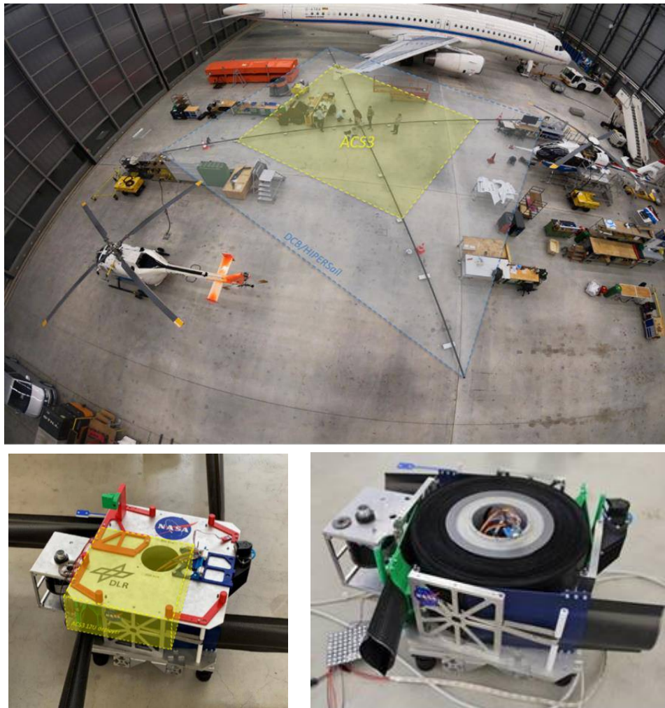
Figure 21. Joint NASA-DLR 16.5-meter booms, 520 m 2 , 27U-scaled DCB “HIPERSail” solar sail system engineering development unit. The 12U-scaled ACS3 7.0-m boom, 80 m 2 solar sail technology demonstrator is shown for scale. Both ACS3 and DCB HIPERSail use similar deployable composite boom technology and deployer architectures. 11
