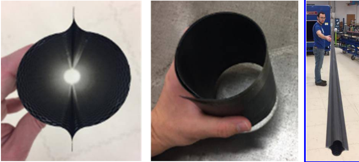
Figure 2. NASA Deployable Composite Boom (DCB) booms. DCB boom technology uses very thin carbon fiber composite plain-weave and unidirectional plies for maximizing the curvature strain tolerance of the boom wall laminates when flattening and rolling for stowage. This enables stowage of very long load-carrying booms in very small volumes in CubeSat form factor spacecraft.
