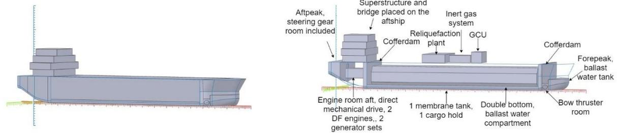
Fig.5: Design solution II (membrane tank, mechanical propulsion system)
