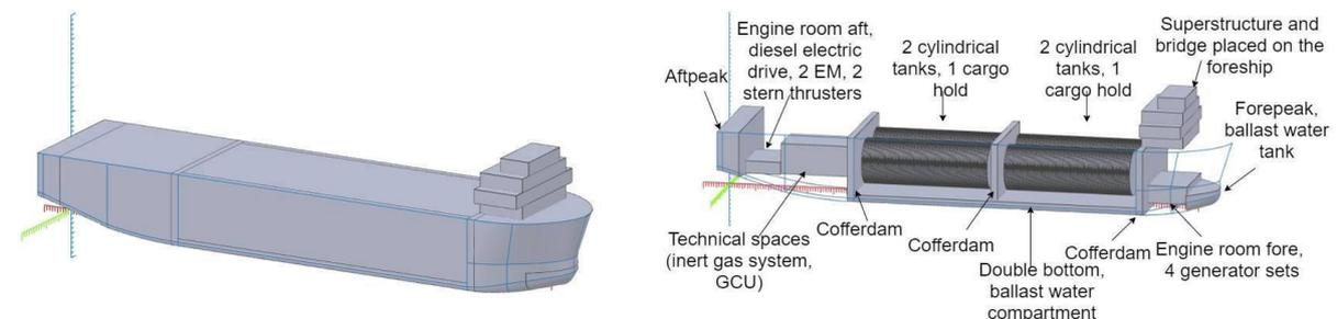
Fig.7: Design Solution IV (cylindrical tanks, diesel-electric propulsion system)
