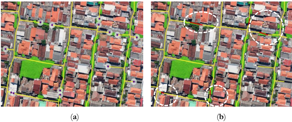
Figure 3.8 Road centerline completion by a tree-constrained extended dangle method. (a) A missing centerline segment is identified as non-empty intersection between tree polygon (green) and the dangle polygon (white circle) of a dangle point (purple); (b) road gap filling adds new road segments (red lines inside dotted white circles) forming a complete road centerline.
