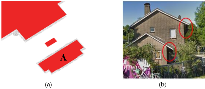
Figure 5.13 Comparison of Bag building polygon (red) and the AHN3 building points (grey) in case of overhanging roof. (a) Top view building definition of BAG polygon (red) and the AHN3 building points (grey); (b) Building “A” has overhanging roof (red circle) ©GoogleStreetView.
