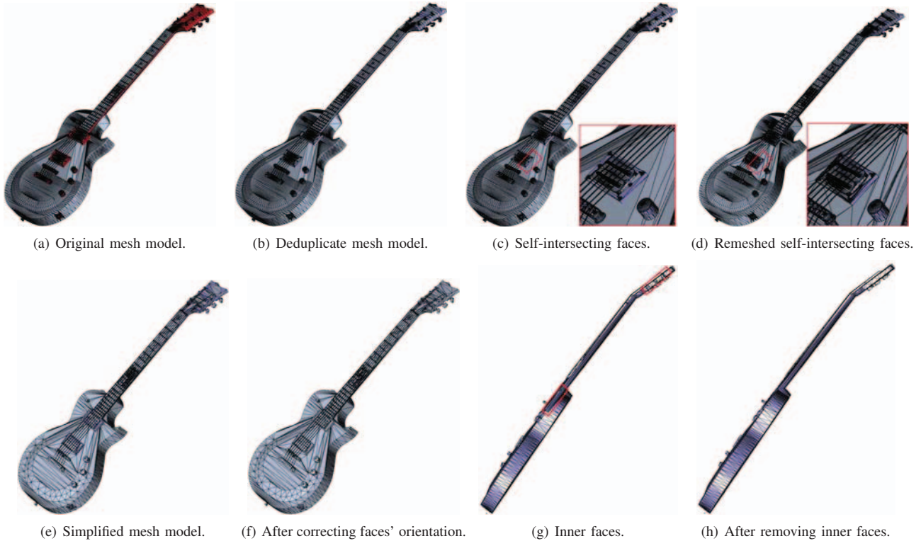
Fig. 2. Visualization of the intermediate processing results for guitar_0205 in ModelNet40 [8] dataset. Gray face indicates outside and light blue face indicates inside. Processing sequence: (a) Original mesh model ( red part is duplicate elements ). (b) Mesh model processed via f_{dedup} , f_{remove\_deg} and f_{remove\_iso} . Light blue face means its orientation is incorrect. (c) A local patch of self-intersecting faces. (d) Self-intersecting faces are repaired by remeshing self-intersections algorithm. (e) We simplify the mesh model to speed up the processing of subsequent steps. (f) Mesh model of previous steps exists wrong face orientation, which is corrected via Algorithm 1 . (g) A cross-section view of the model to reveal its inner structure. (h) A cross-section view of the model after removing inner faces, which proves that we can remove the inner faces thoroughly.
