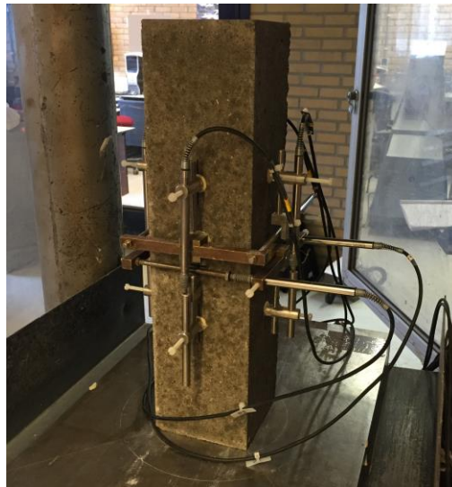
Figure 6.1 Testing set-up for elastic modulus measurement on AAS and AASF concrete.
