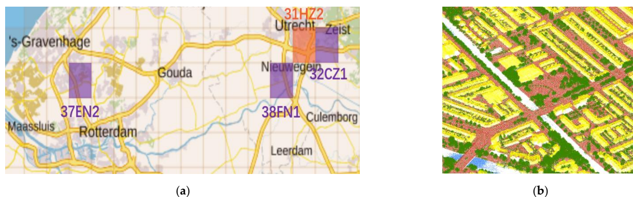
Figure 6. Dutch up-to-date Elevation Archive File, version 3 (AHN3) grids selected for this study. (a) Grids in purple are used as training while the grid in orange was used as the test area; (b) AHN3 point clouds labeled as bare land (brown), buildings (yellow), water (blue), and “others” (green).
