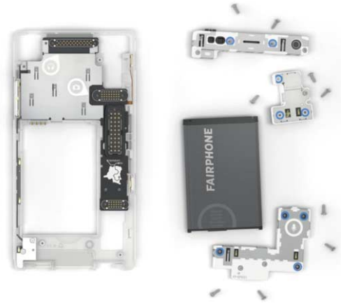
Figure 2. Internal modules of the Fairphone 2.
