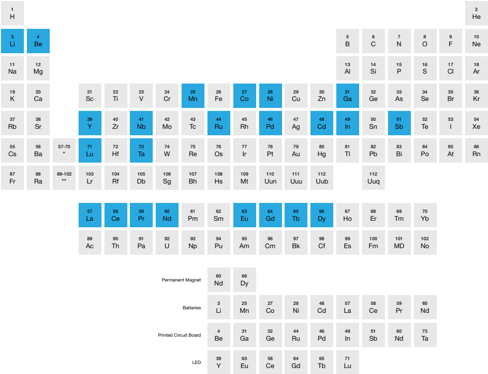
Figure 19. Examples of components and related CRM's in wind turbines. Developed from (CRM_Innonet 2013) and (CRM_InnoNet, 2015). Published in Critical Raw Materials, Circular Economy and Wind Turbines, Fromberg, et al, 2015.
