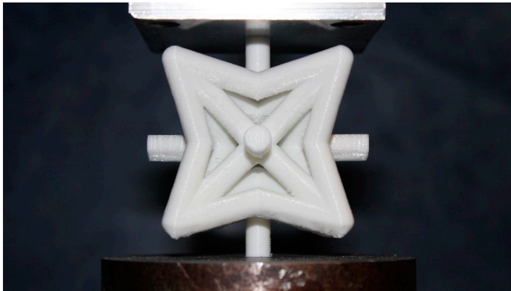
Figure 8. An additively manufactured specimen with \mu = 0.25 under loading test.
