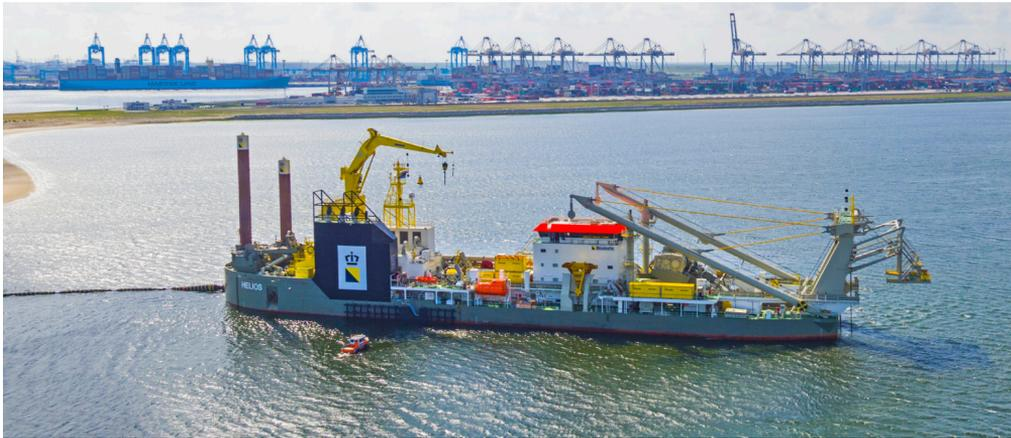
Figure 1.3: The self-propelled cutter suction dredger "Helios" owned by Royal Boskalis Westminster N.V. Source: Boskalis (2017)
