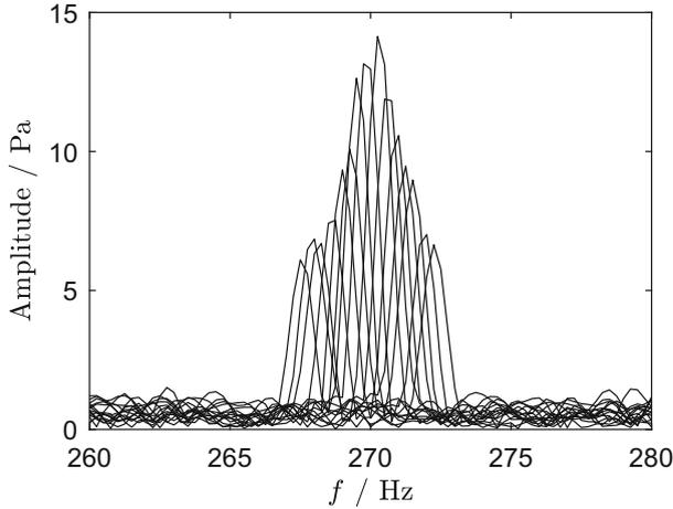
**Fig. 2.** Mode  $k = 2$  acoustic resonance.
