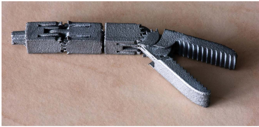
Fig. 1. Rolling toothed joint fabricated by AM.
