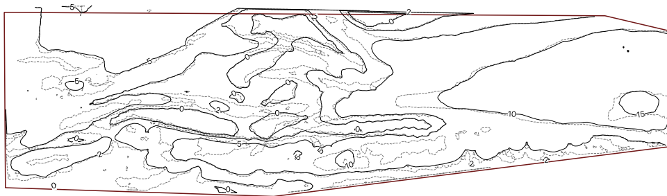
Figure 5. Originally extracted isobaths from TIN (grey) and the generalised isobaths for a scale of 1:100k (black). Notice how lines are smoothed, peaks are aggregated, irrelevant details omitted.
