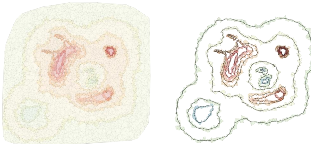
a) Triangulation coloured on interval (TRG nodes) b) TRG edges with extracted isobaths
