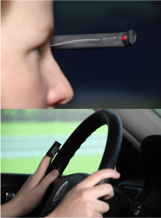
Figure A2. The head-mounted PDT headband with the red LED and the micro switch.
