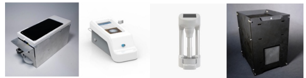
Fig. 3. Mobile phone and Raspberry Pi based Schistoscopes.
