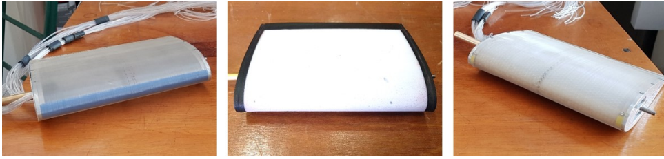
Figure 3.6: Pictures of the solid (on the left), melamine (in the middle), and porous airfoils (on the right) manufactured at VKI.
