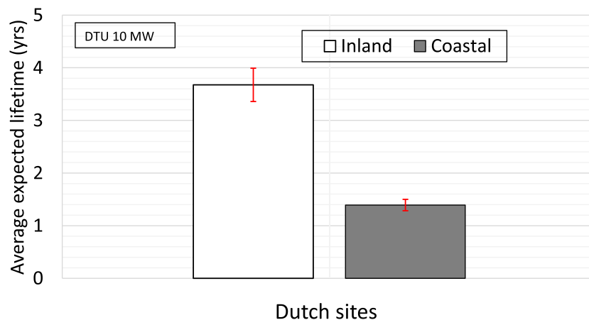
FIGURE 16 Comparison of average erosion lifetime for WTB at inland and coastal sites
