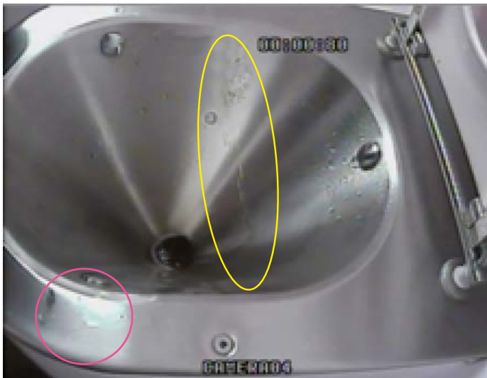
Figure 5.10 Close-up recording of the toilet bowl, in which urine spillage (in pink circle) is visible. The urine stream appears in the yellow oval.
