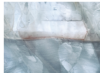
FIG. 15 Left, middle, right: Tomorrow-Element contamination / Algae formation through condensation in the cells
