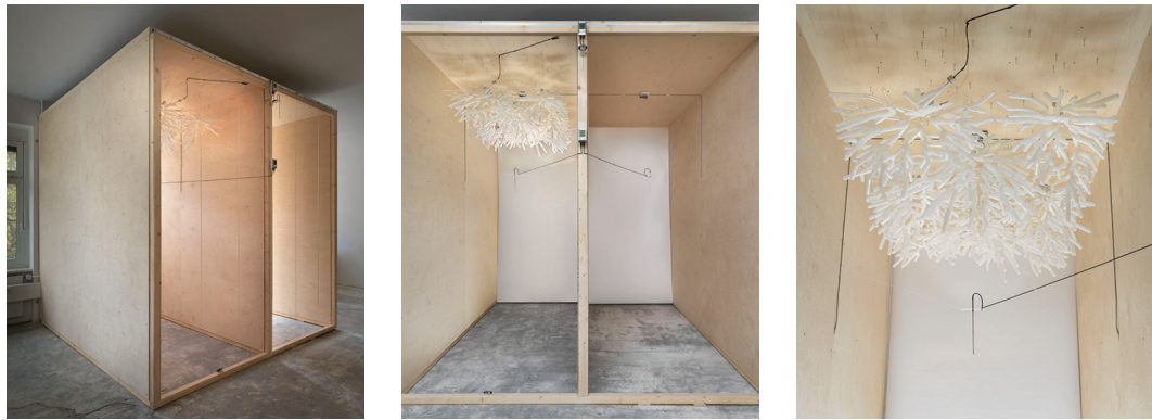
FIG. 11 Experimental set-up for thermal cycling of dendritic prototypes showing twin test cells (left), placement of measurement probes (middle) and dendritic structure (right)
