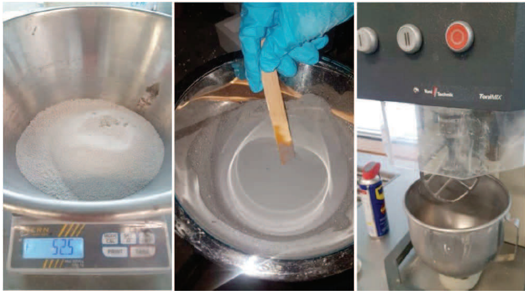
FIG. 9 Preparation of a water-proof expanded glass/water glass mixture; standard formulation: slurry consisting of two parts by weight water glass (potassium silicate) and one part powdery, mineral hardener; ratio of slurry/expanded glass approx. 80/20, drying at approx. 150°C.
