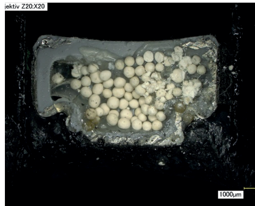
FIG. 2 Spacers enlarged 20 times
