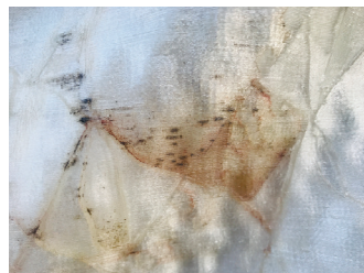
FIG. 15 Left, middle, right: Tomorrow-Element contamination / Algae formation through condensation in the cells
