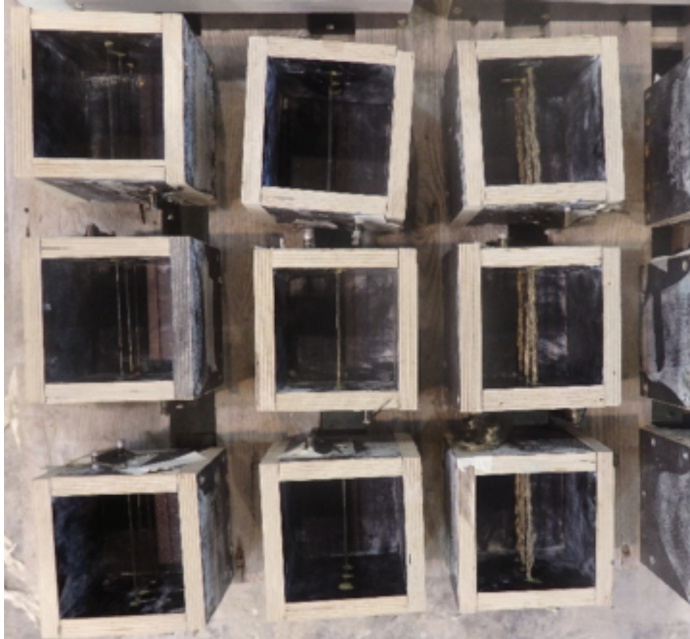
FIG. 7 Single rovings in form-work for pull-out tests
