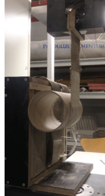
FIG. 8 Single-layer basalt fabric, test setup – peel-off test
