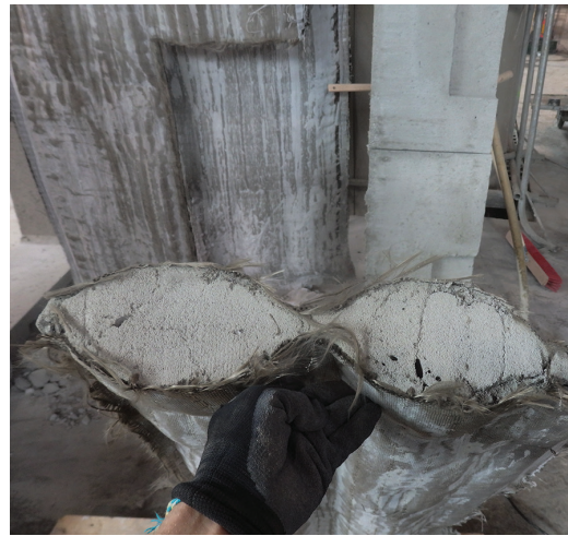
FIG. 18 In the background, large-format basalt fabric, foamed with cement foam, height 3.80 m, section of the element in front
