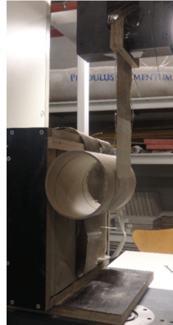
FIG. 8 Single-layer basalt fabric, test setup – peel-off test
