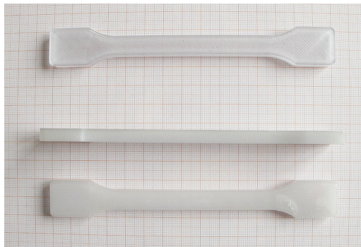
FIG. 3 3D printed test specimen tensile test
