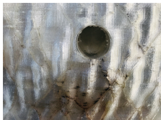
FIG. 15 Left, middle, right: Tomorrow-Element contamination / Algae formation through condensation in the cells
