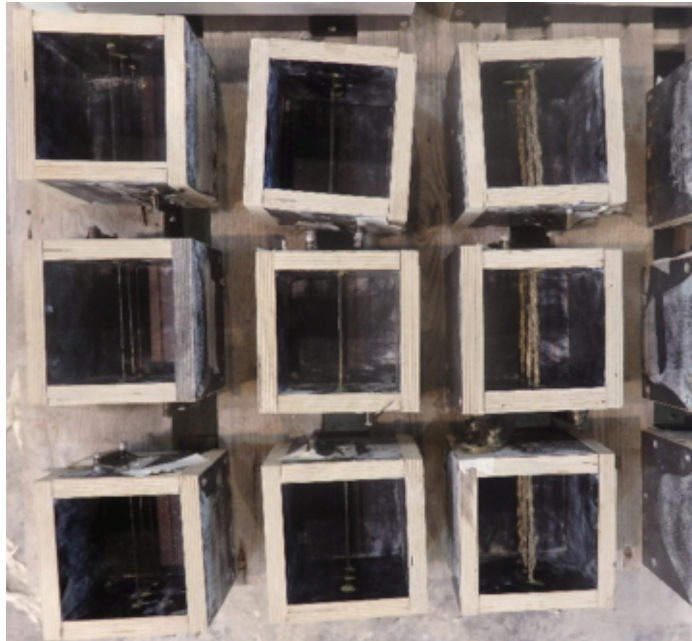
FIG. 7 Single rovings in form-work for pull-out tests
