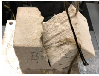
FIG. 11 Pull-out test to determine the adhesion of basalt roving / cementitious foam
