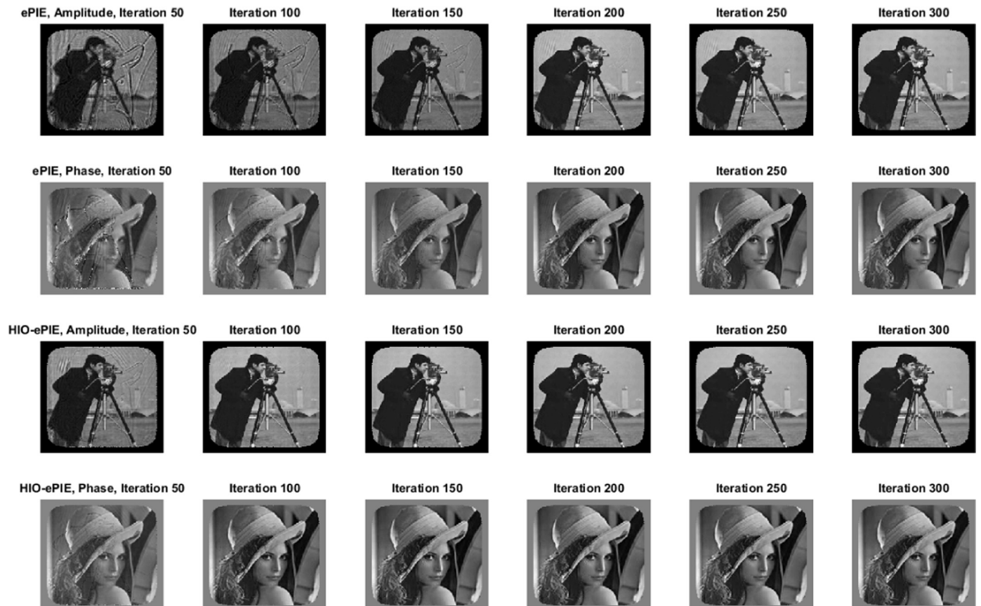
Fig. 9. Reconstruction for ePIE and HIO-ePIE in the noise-free case, with 8 \times 8 small probes.
