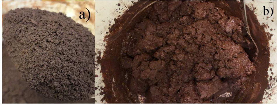
Figure 3-13. Forming large agglomerates after adding 4% extra moisture content; a) MC_{as,rec} , b)
