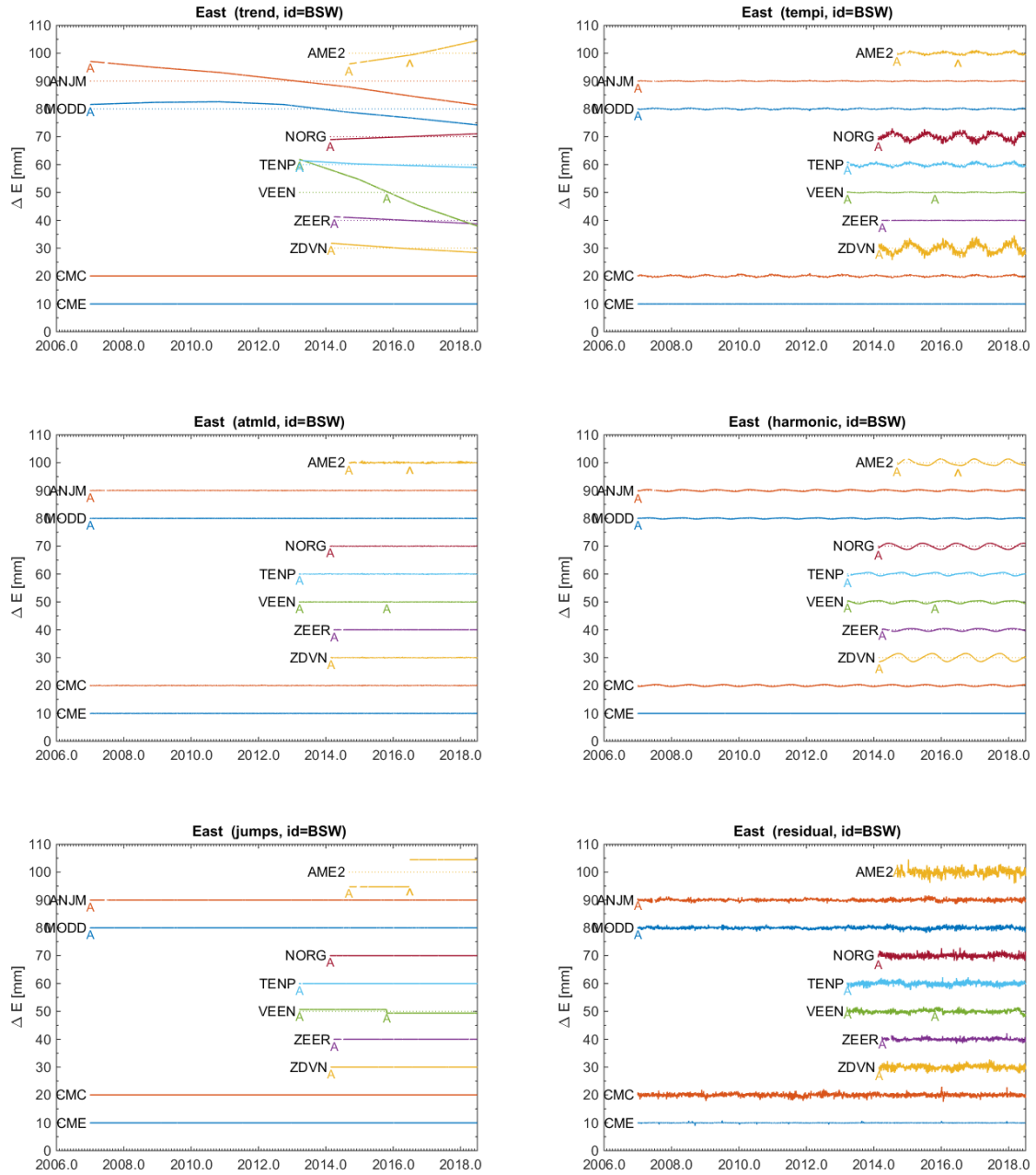
Figure 5.2: East time series components for selected NAM monitoring stations. From left to right, top to bottom, a) estimated trend function, b) temperature influence, c) atmospheric loading, d) annual and semi-annual harmonics, e) steps and f) residuals after fit. Data from 8 selected stations is shown using results from the decomposition of the Bernese GNSS Software (BSW) time series. Antenna changes are indicated by a “A”, other steps by a “^”. The series marked by CMC is the common mode correction estimated from the previous iteration, which is the same for every station. The series marked by CME is the common mode estimated during this iteration. The common modes have been computed from more stations than shown in this figure. The original time series (not shown) is the sum of the station time series in each plot, with the CME and CMC components added.
