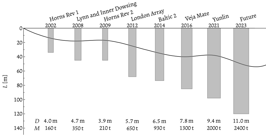
Figure 1.2: Increasing dimensions of monopile foundations for offshore wind over the past two decades. L represents the length of the pile, D denotes the outer diameter at the lower end of the pile and M is the mass of the pile in metric tons. Adapted from Niess (2013), Boskalis (2016) and Nordenham (2019, June 11).
