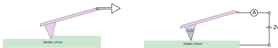
FIGURE 7 | Dry lithiation methods. Left: mechanical lithiation. Right: electrochemical alloying method.
