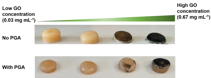
Figure S4.1 Side view of BC-GO composites obtained by in situ fermentation. Without PGA, the sample thickness decreases at higher GO concentration in fermentation medium. After the addition of PGA, the sample thickness remains similar at various GO concentrations. GO could penetrate into the BC network (black area) only at higher GO concentrations.
