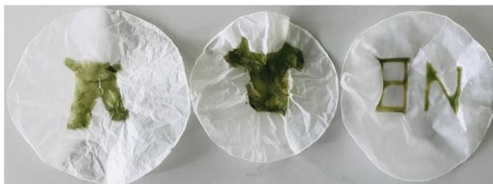
Figure S6.12 Stability of bioprints. Photographs of bioprinted microalgae on bacterial cellulose following 1 month of incubation under ambient conditions.
