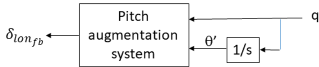
Figure 8.2-3: Perturbation and Sweep Method for Determining the Feedback Response from a SIMLINK Block Diagram.
