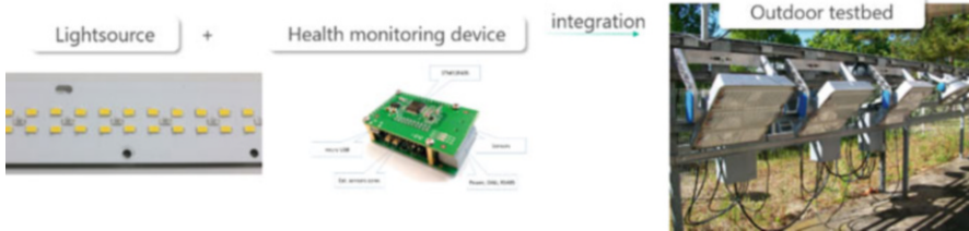
Fig. 13.25 System integration into an outdoor test bed
