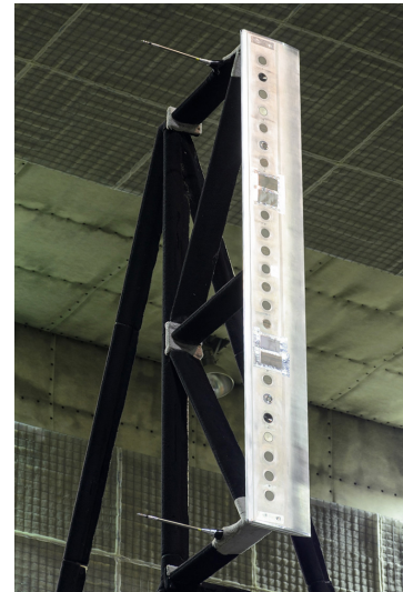
Figure 4. In-flow microphone wing.
