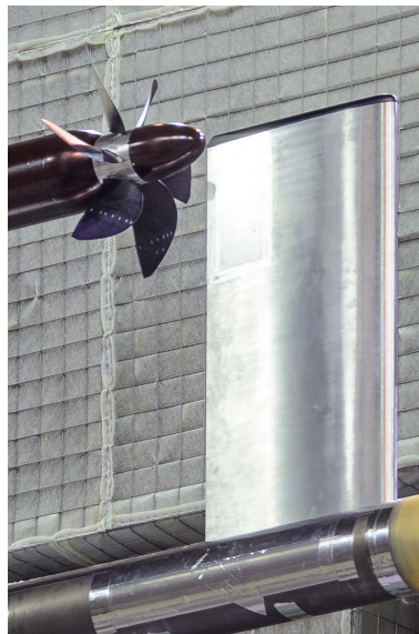
Figure 2. APIAN propeller installed downstream of the pylon model.
