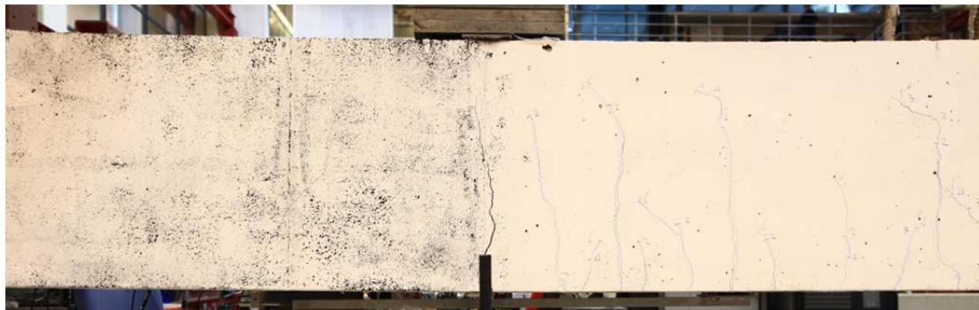
Fig. 5.97.1. Crack pattern after failure north side
