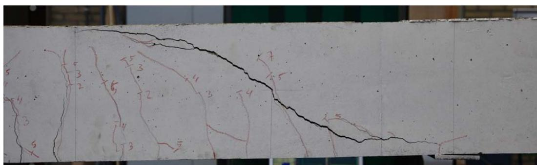
Fig. 5.28.2. Crack pattern after failure south side
