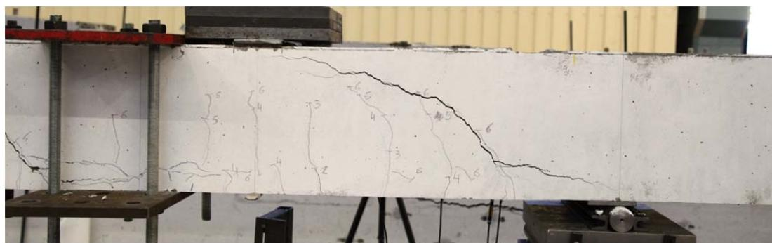
Fig. 5.7.2. Crack pattern after failure south side
