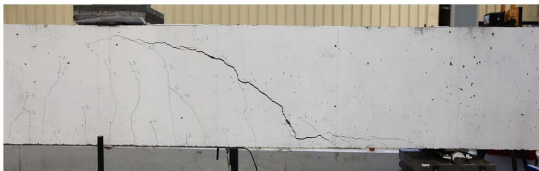
Fig. 5.46.2. Crack pattern after failure south side
