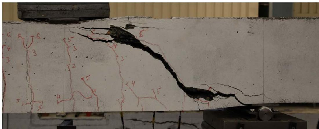
Fig. 5.33.2. Crack pattern after failure south side
