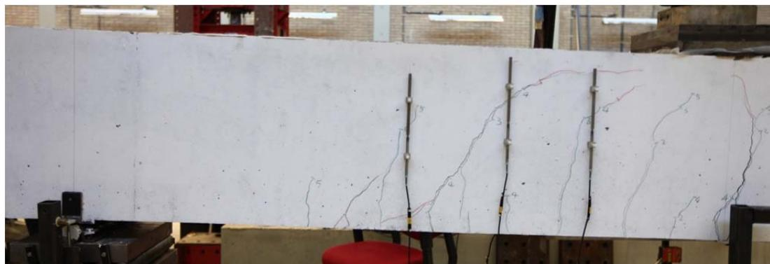
Fig. 5.42.1. Crack pattern after failure north side
