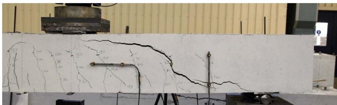
Fig. 5.3.2. Crack pattern after failure south side
