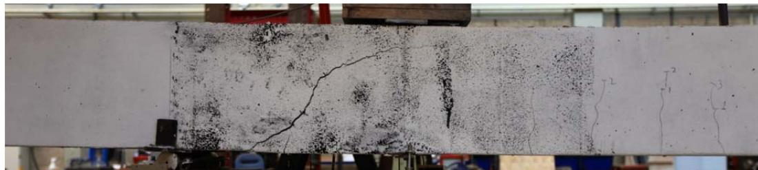
Fig. 5.75.1. Crack pattern after failure front side
