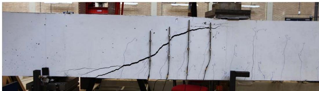
Fig. 5.44.1. Crack pattern after failure north side
