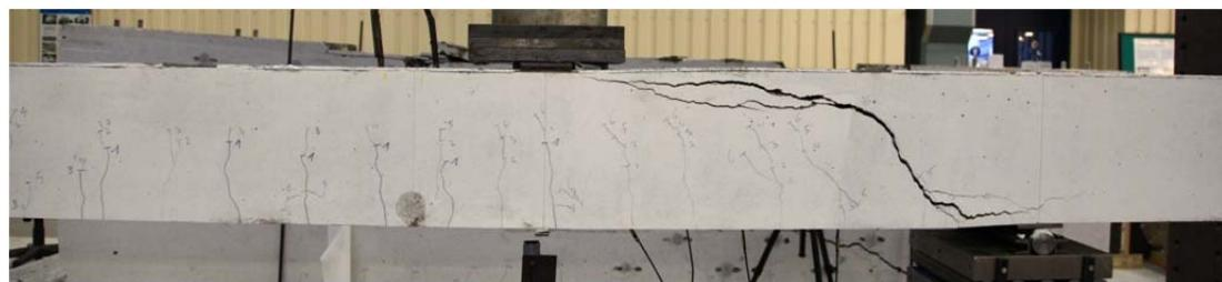
Fig. 5.6.2. Crack pattern after failure south side
