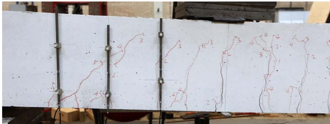
Fig. 5.67.1. Crack pattern after failure north side
