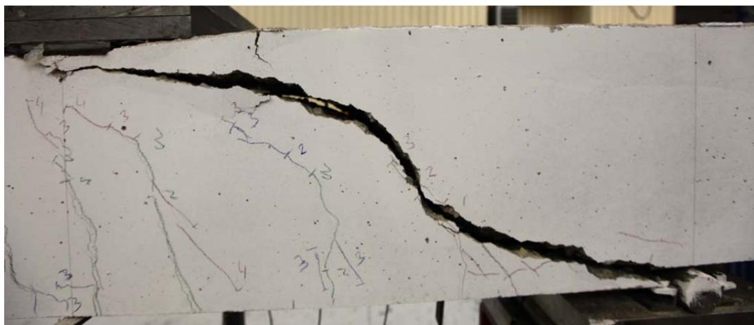
Fig. 5.64.2. Crack pattern after failure south side
