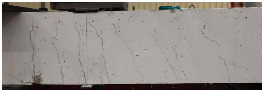
Fig. 5.69.2. Crack pattern after failure south side
