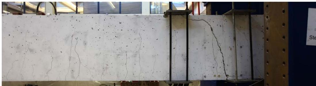
Fig. 5.86.3. Shear failure at A-side
