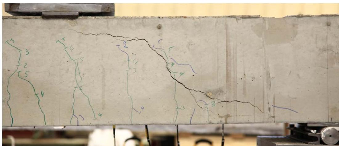
Fig. 5.23.2. Crack pattern after failure south side
