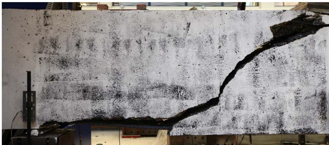
Fig. 5.100.1. Crack pattern after failure north side
