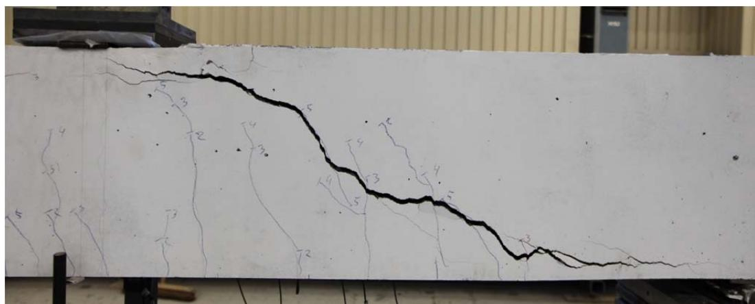
Fig. 5.44.2. Crack pattern after failure south side
