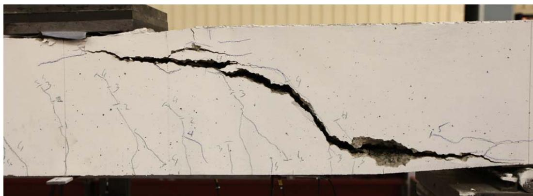
Fig. 5.59.2. Crack pattern after failure south side
