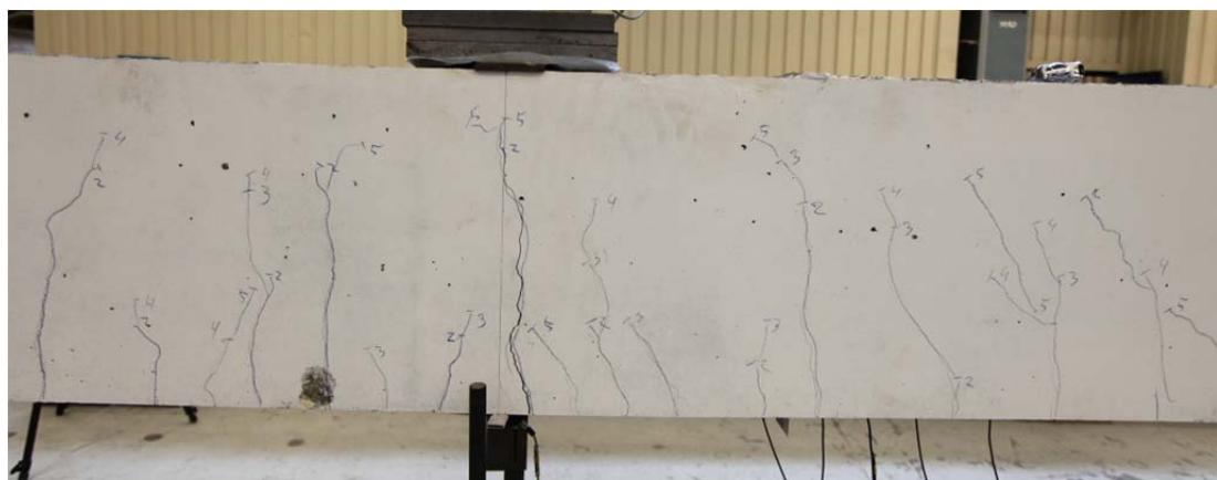
Fig. 5.43.2. Crack pattern after failure south side
