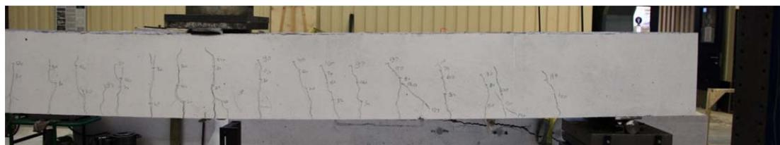
Fig. 5.1.2. Crack pattern after failure south side
