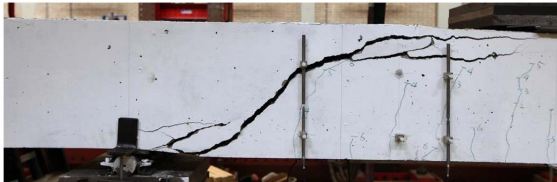
Fig. 5.8.1. Crack pattern after failure north side
