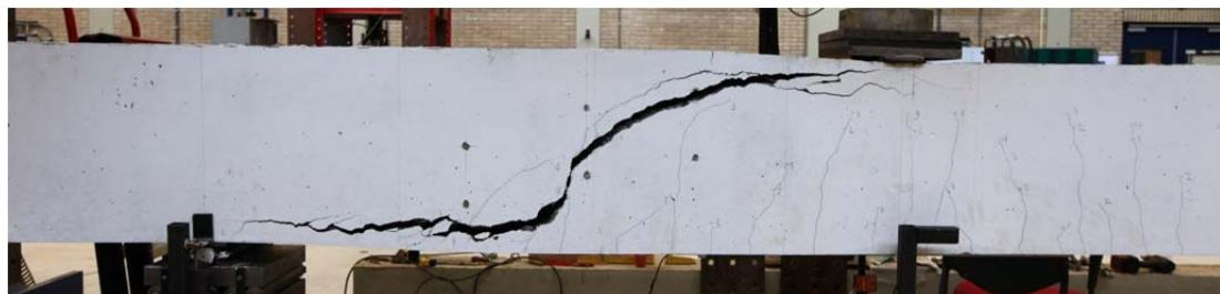
Fig. 5.49.1. Crack pattern after failure north side
