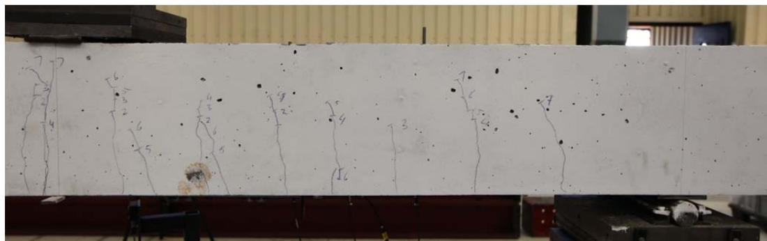
Fig. 5.10.2. Crack pattern after failure south side
