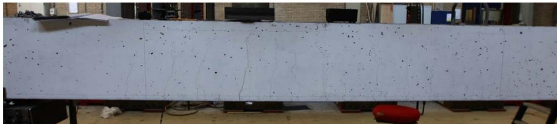
Fig. 5.82.1. Crack pattern after failure north side
