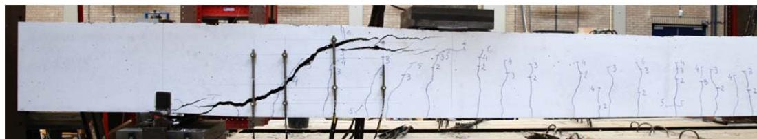
Fig. 5.17.1. Crack pattern after failure north side
