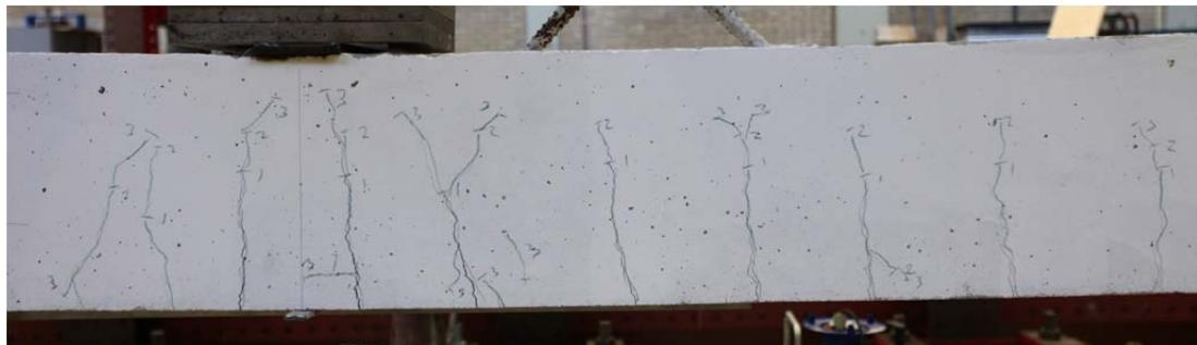
Fig. 5.62.1. Crack pattern after failure north side
