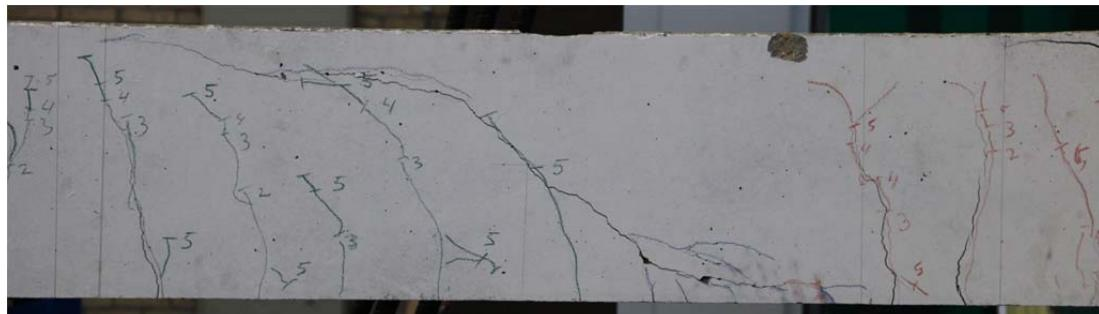
Fig. 5.27.2. Crack pattern after failure south side
