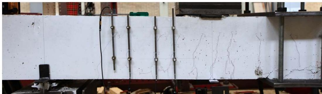
Fig. 5.69.1. Crack pattern after failure north side
