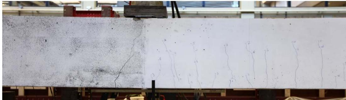
Fig. 5.78.1. Crack pattern after failure front side
