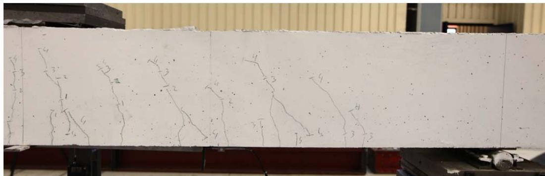
Fig. 5.58.2. Crack pattern after failure south side
