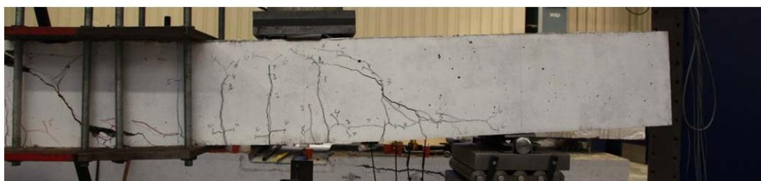
Fig. 5.34.2. Crack pattern after failure south side
