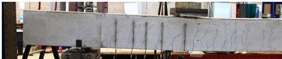
Fig. 5.13.1. Crack pattern after failure north side
