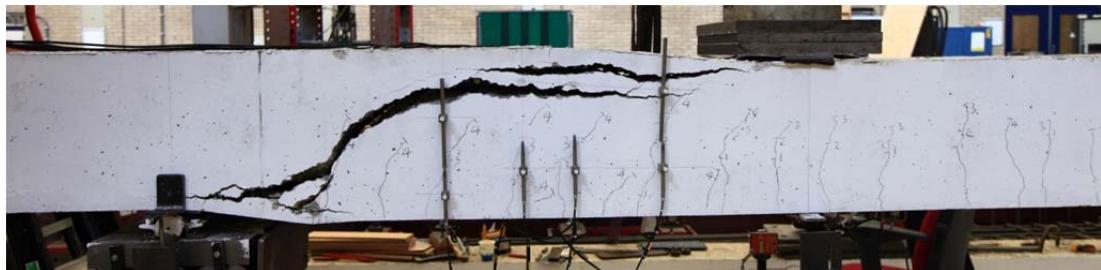
Fig. 5.57.1. Crack pattern after failure north side
