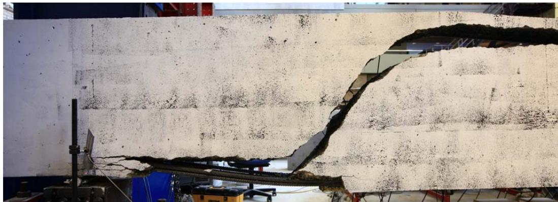
Fig. 5.104.1. Crack pattern after failure at east side of beam
