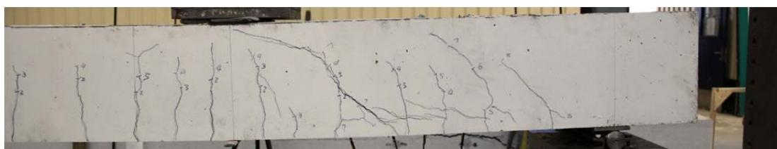
Fig. 5.4.2. Crack pattern after failure south side
