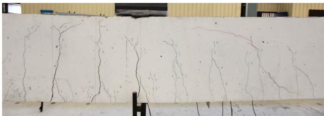
Fig. 5.42.2. Crack pattern after failure south side
