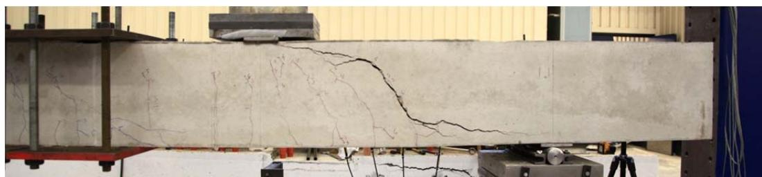
Fig. 5.25.2. Crack pattern after failure south side
