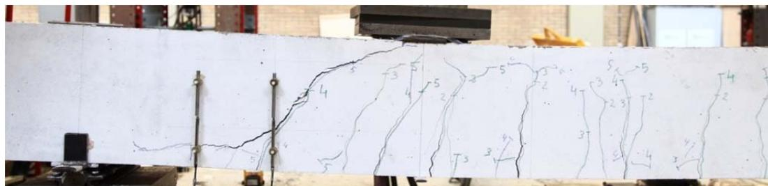
Fig. 5.32.1. Crack pattern after failure north side
