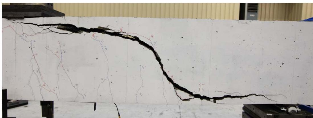
Fig. 5.52.2. Crack pattern after failure south side
