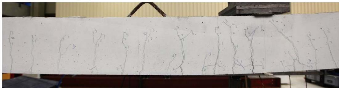
Fig. 5.63.2. Crack pattern after failure south side
