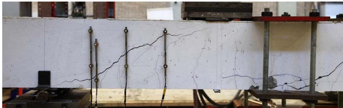
Fig. 5.7.1. Crack pattern after failure north side
