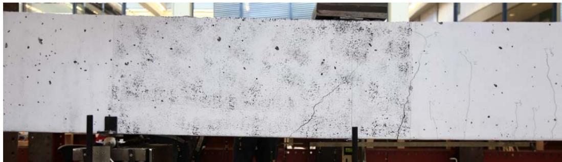
Fig. 5.81.1. Crack pattern after failure front side
