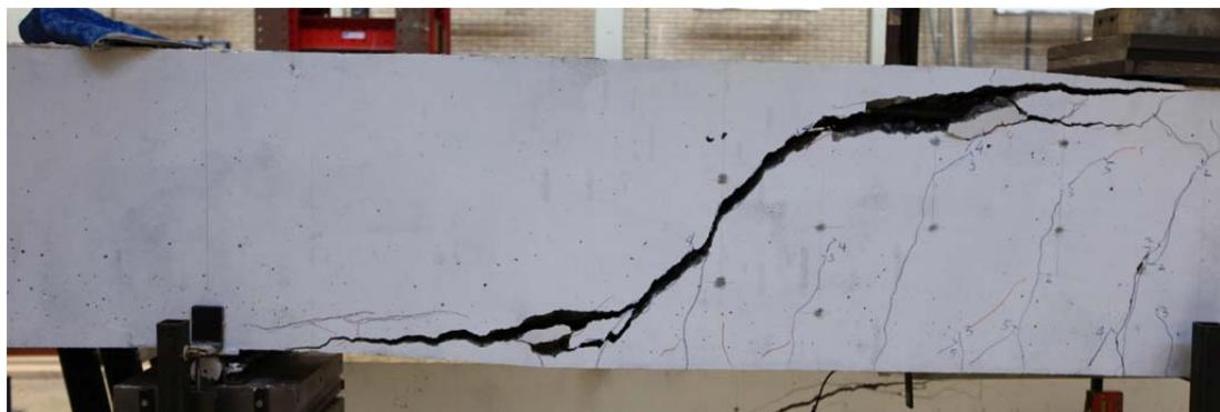
Fig. 5.52.1. Crack pattern after failure north side
