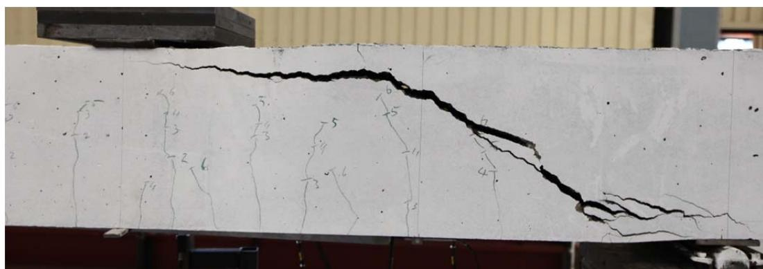
Fig. 5.8.2. Crack pattern after failure south side
