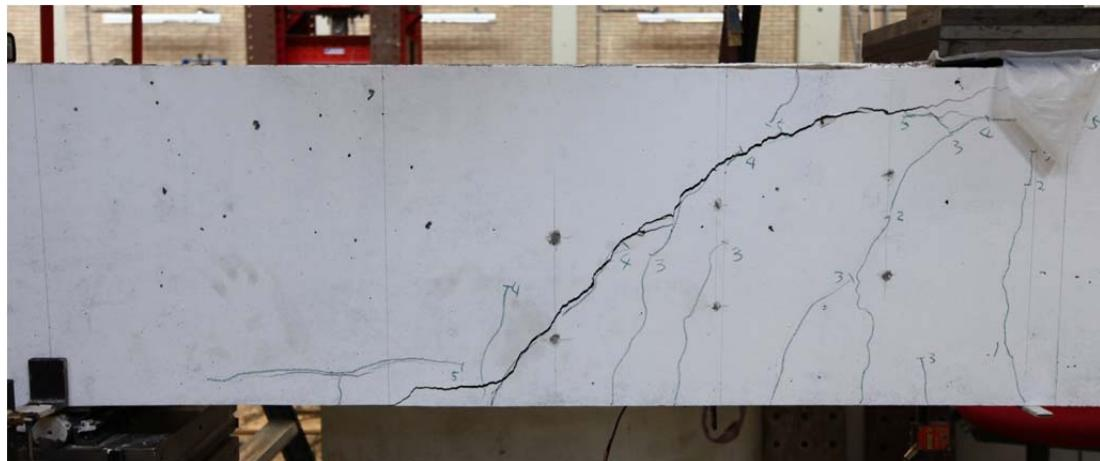
Fig. 5.46.1. Crack pattern after failure north side
