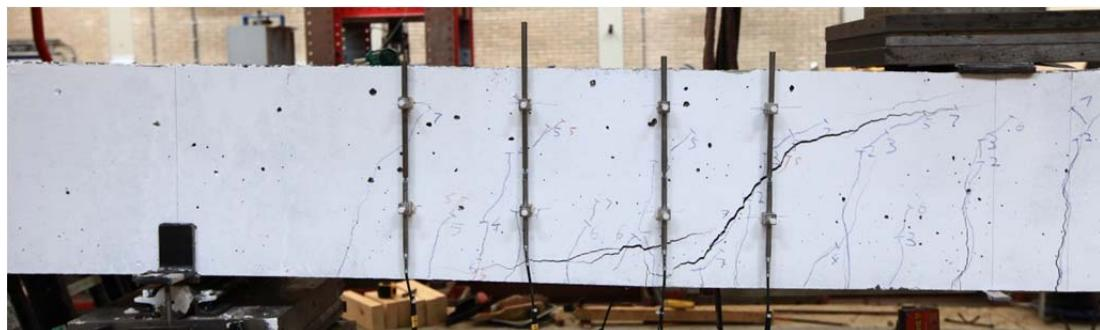
Fig. 5.11.1. Crack pattern after failure north side
