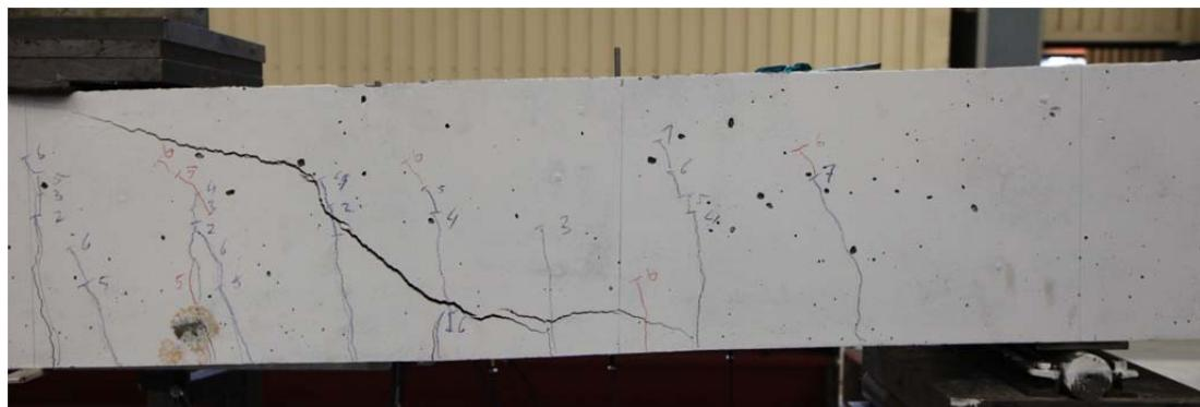
Fig. 5.11.2. Crack pattern after failure south side
