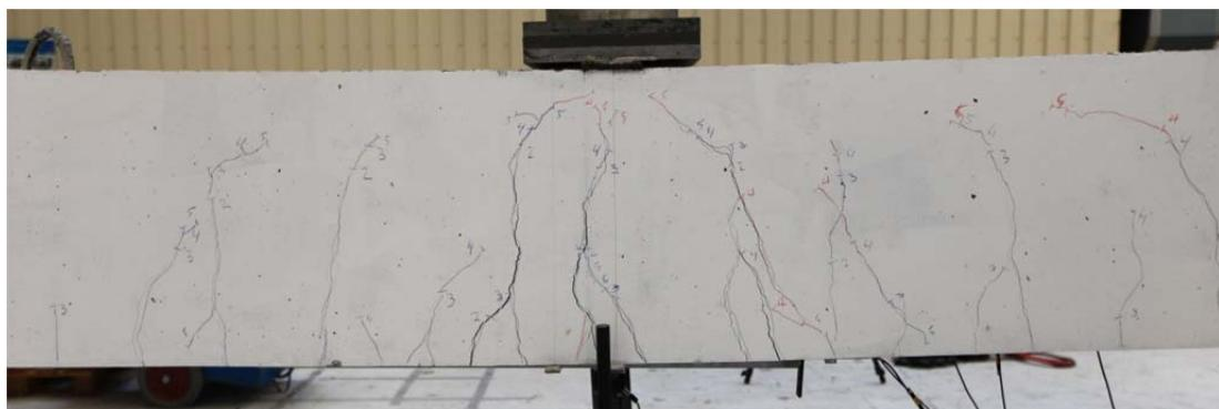
Fig. 5.51.2. Crack pattern after failure south side
