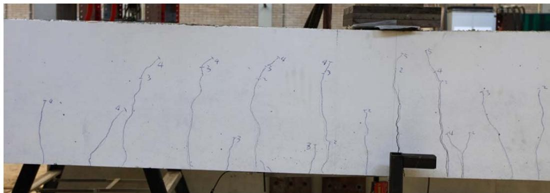
Fig. 5.47.1. Crack pattern after failure north side
