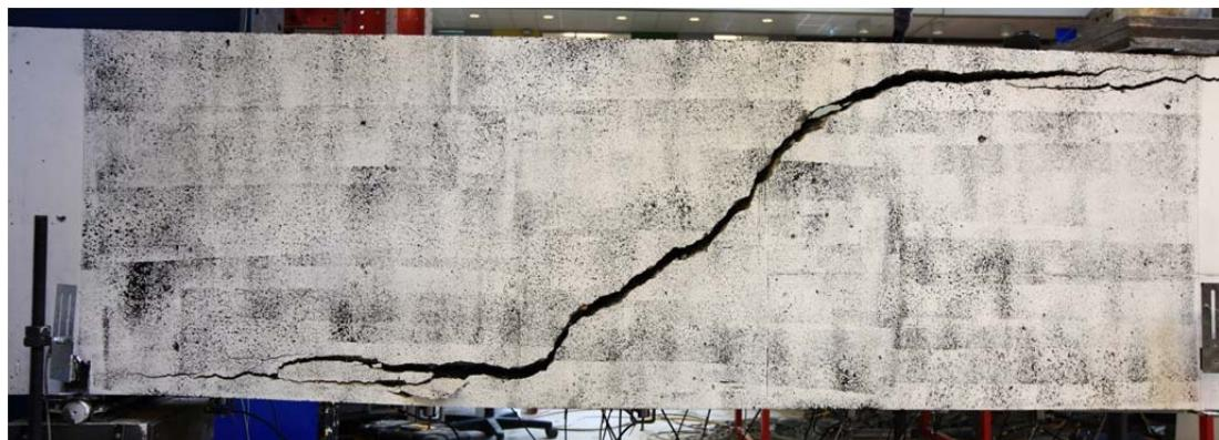
Fig. 5.94.1. Crack pattern after failure east side
