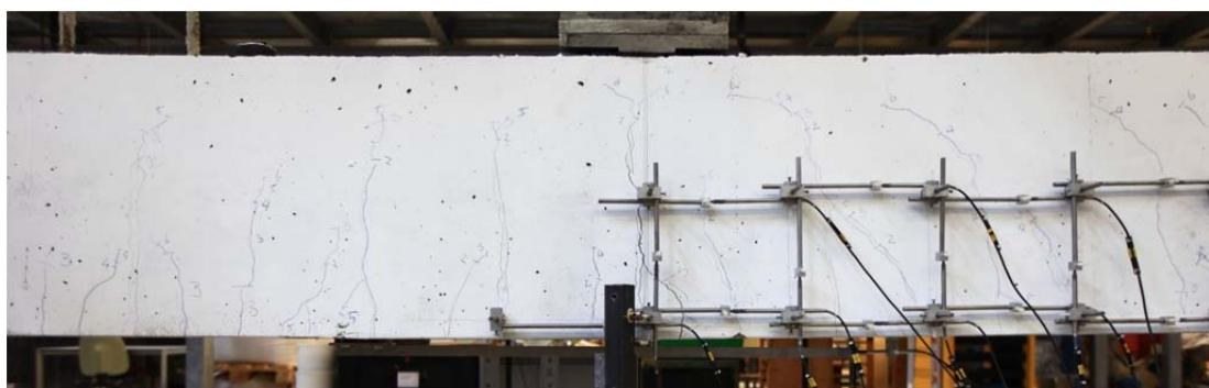
Fig. 5.97.2. Crack pattern after failure south side
