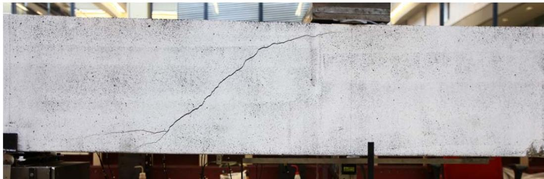
Fig. 5.77.1. Crack pattern after failure front side
