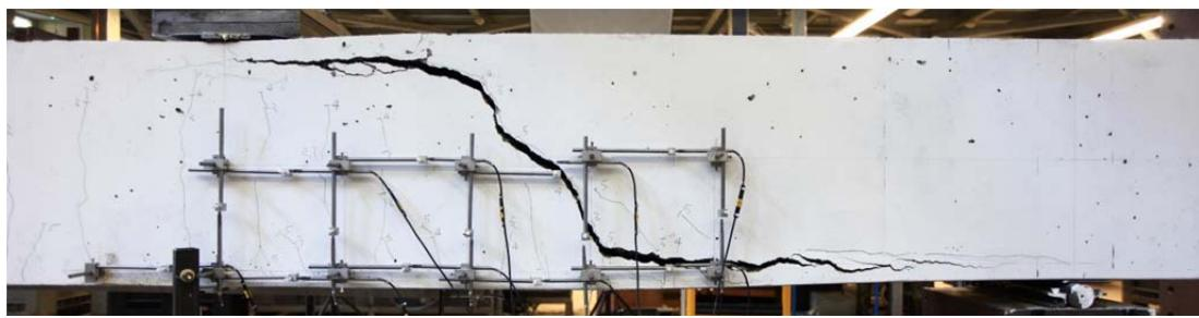
Fig. 5.99.2. Crack pattern after failure west side
