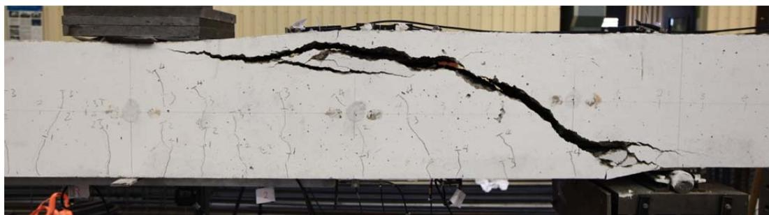
Fig. 5.57.2. Crack pattern after failure south side
