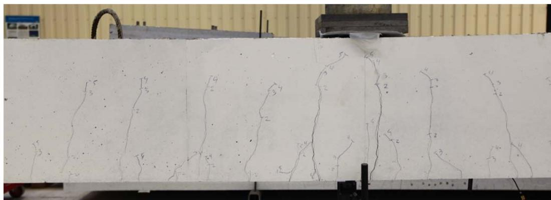
Fig. 5.47.2. Crack pattern after failure south side
