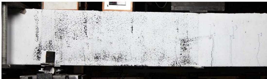
Fig. 5.71.1. Crack pattern after failure north side
