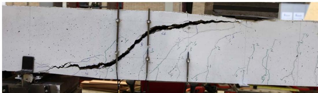
Fig. 5.59.1. Crack pattern after failure north side
