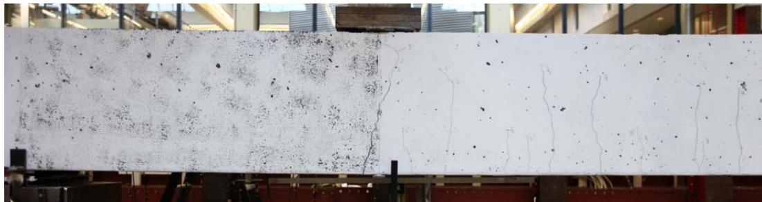
Fig. 5.80.1. Crack pattern after failure front side
