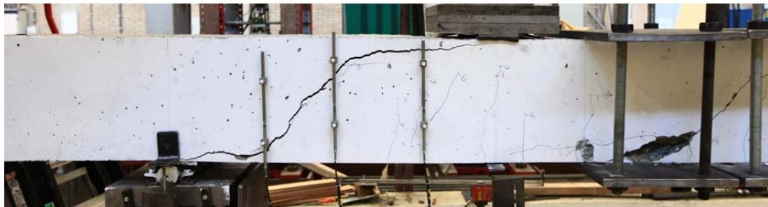
Fig. 5.9.1. Crack pattern after failure north side
