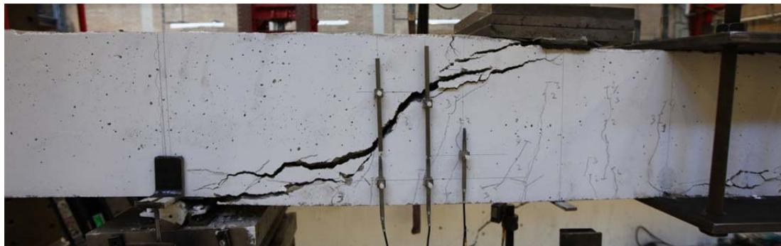
Fig. 5.65.1. Crack pattern after failure north side
