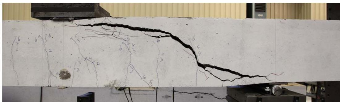
Fig. 5.21.2. Crack pattern after failure south side
