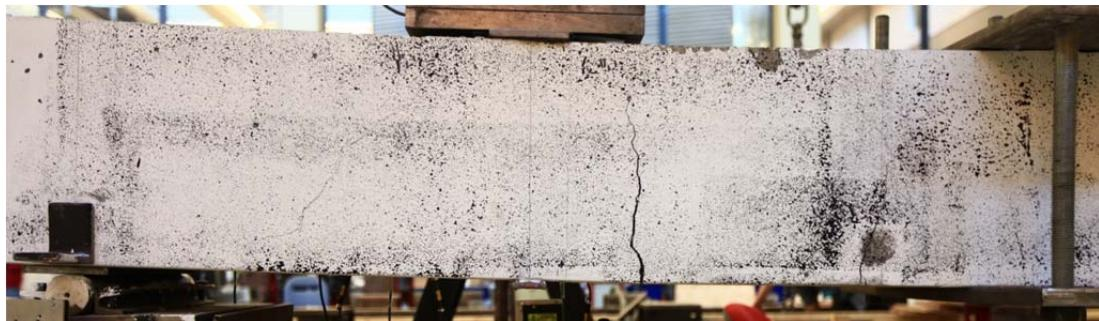
Fig. 5.74.1. Crack pattern after failure front side
