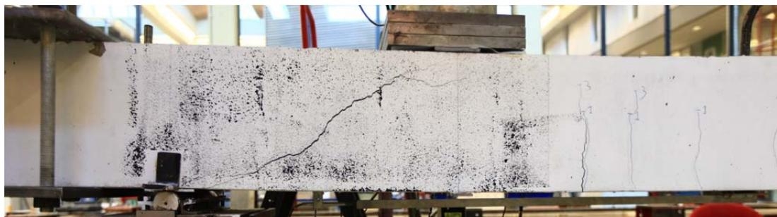
Fig. 5.72.1. Crack pattern after failure front side
