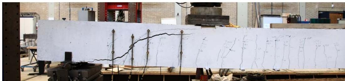
Fig. 5.3.1. Crack pattern after failure north side
