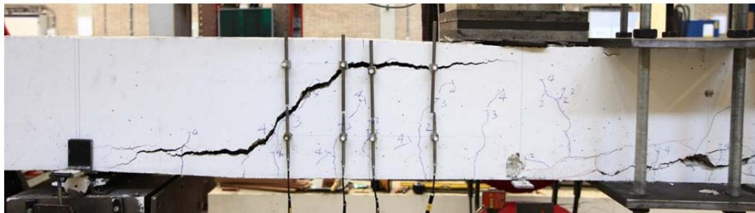
Fig. 5.56.1. Crack pattern after failure north side
