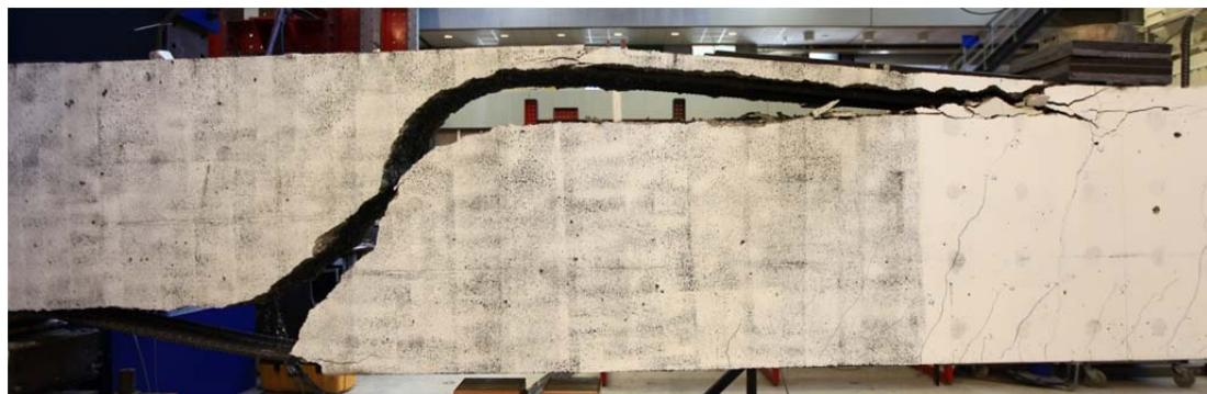
Fig. 5.107.1. Crack pattern after failure at east side of beam
