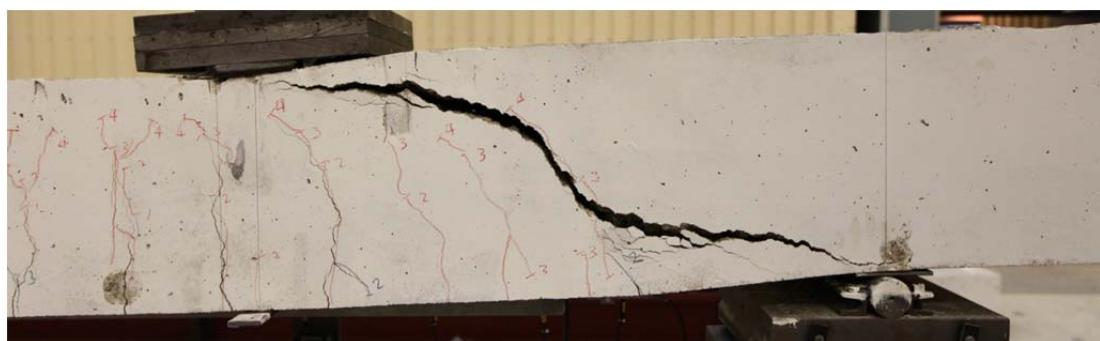
Fig. 5.68.2. Crack pattern after failure south side
