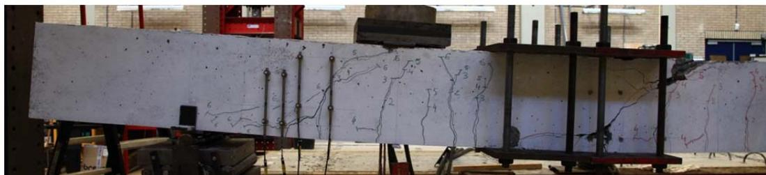
Fig. 5.34.1. Crack pattern after failure north side
