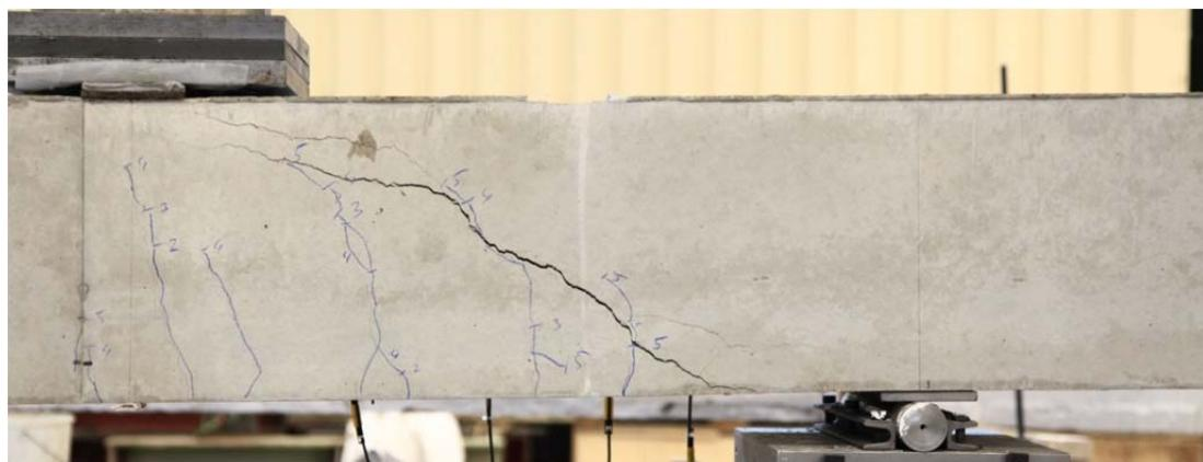
Fig. 5.24.2. Crack pattern after failure south side
