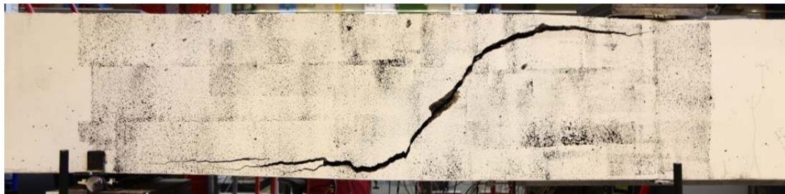
Fig. 5.99.1. Crack pattern after failure east side
