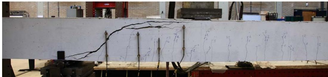
Fig. 5.6.1. Crack pattern after failure north side
