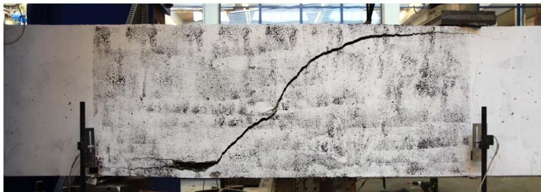
Fig. 5.89.1. Crack pattern after failure north side
