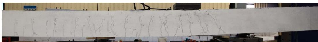
Fig. 5.35.2. Crack pattern after failure south side
