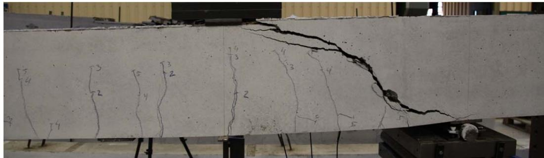
Fig. 5.37.2. Crack pattern after failure south side
