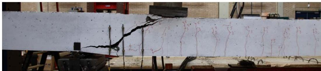
Fig. 5.33.1. Crack pattern after failure north side
