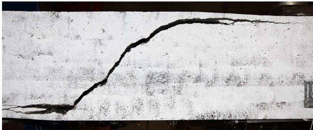
Fig. 5.93.1. Crack pattern after failure east side
