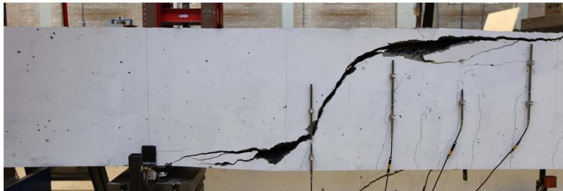
Fig. 5.53.1. Crack pattern after failure north side
