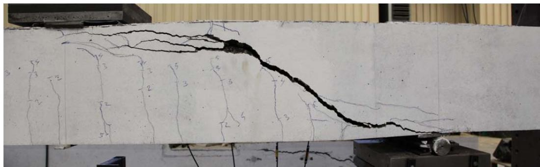
Fig. 5.17.2. Crack pattern after failure south side
