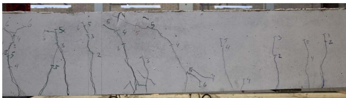
Fig. 5.36.2. Crack pattern after failure south side. (Picture taken after test A602A3.)
