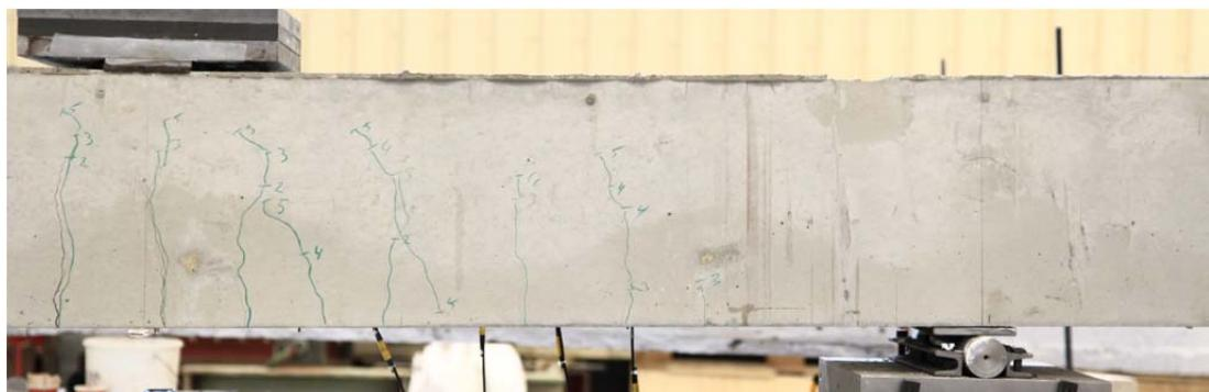
Fig. 5.22.2. Crack pattern after failure south side
