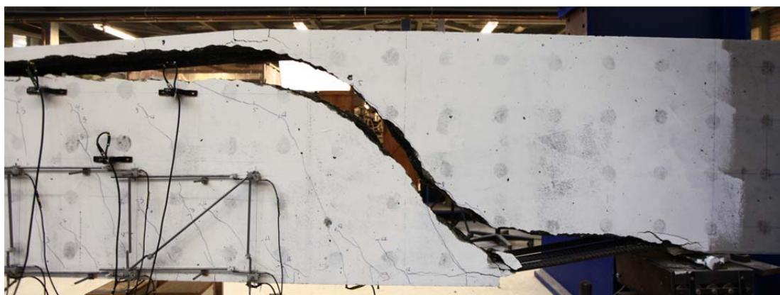
Fig. 5.106.2. Crack pattern after failure and part of LVDT layout at west side of beam
