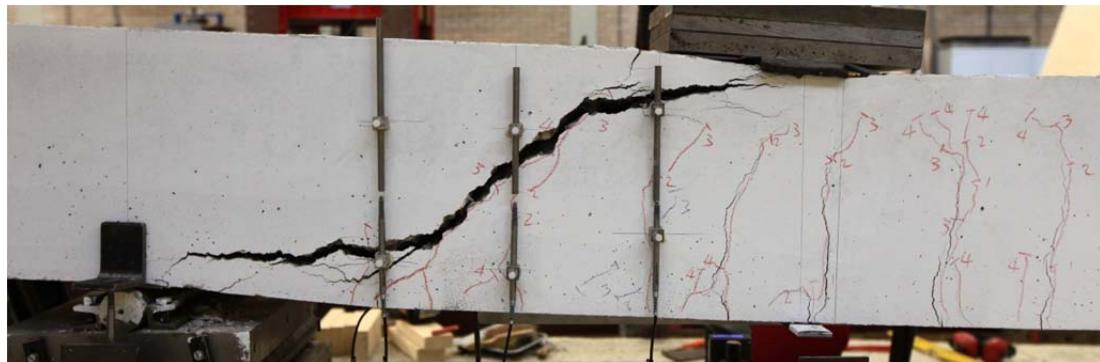
Fig. 5.68.1. Crack pattern after failure north side
