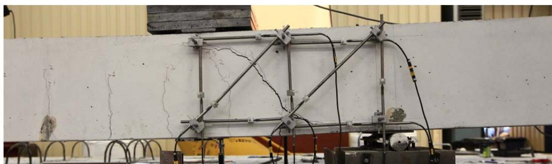
Fig. 5.75.2. Crack pattern after failure back side
