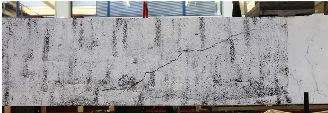
Fig. 5.95.1. Crack pattern after failure north side
