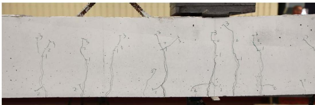
Fig. 5.62.2. Crack pattern after failure south side
