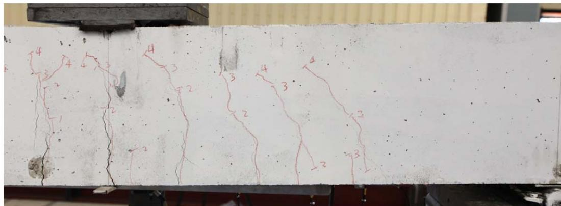
Fig. 5.67.2. Crack pattern after failure south side
