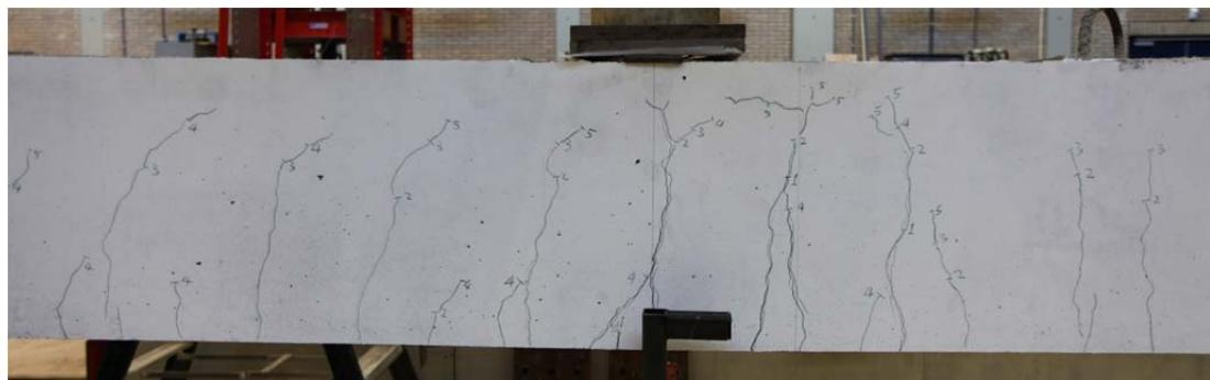
Fig. 5.41.1. Crack pattern after failure north side
