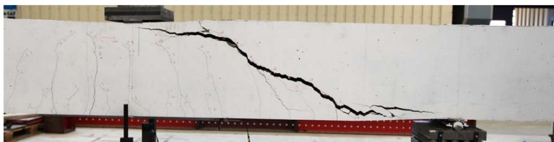
Fig. 5.48.2. Crack pattern after failure south side
