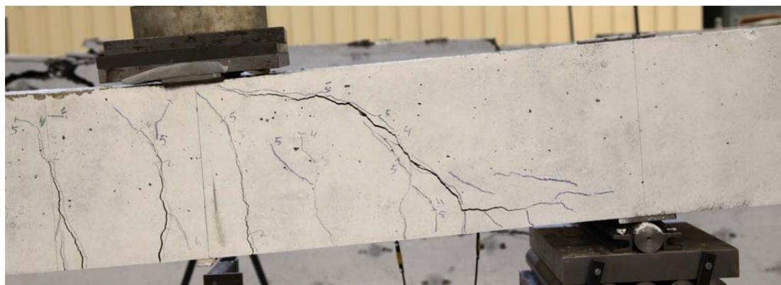
Fig. 5.32.2. Crack pattern after failure south side
