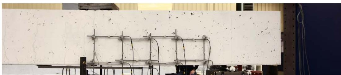
Fig. 5.80.2. Crack pattern after failure back side
