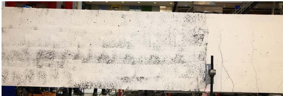
Fig. 5.92.1. Crack pattern after failure east side
