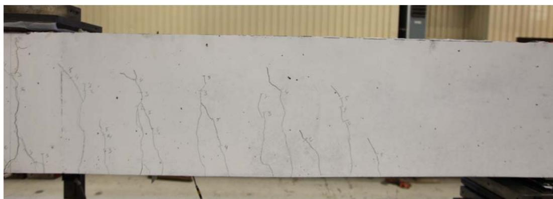
Fig. 5.41.2. Crack pattern after failure south side
