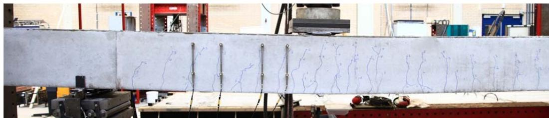
Fig. 5.12.1. Crack pattern after failure north side
