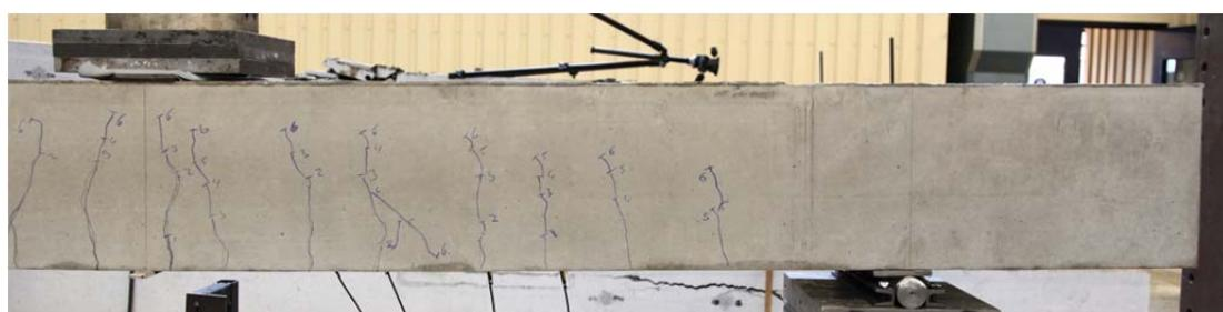
Fig. 5.12.2. Crack pattern after failure south side
