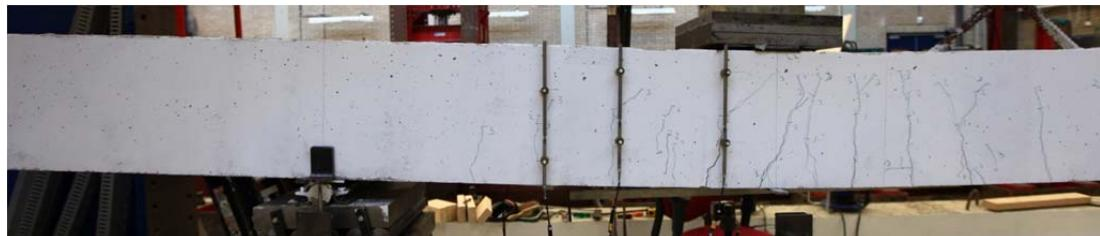
Fig. 5.63.1. Crack pattern after failure north side
