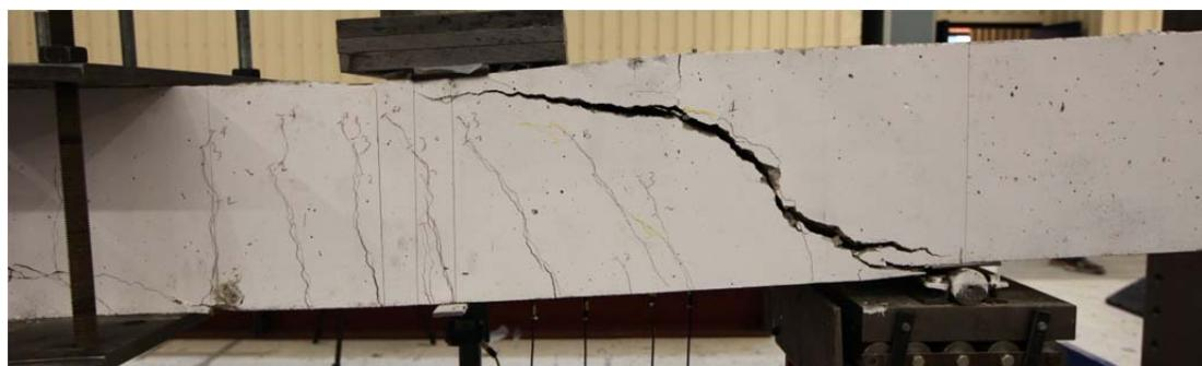
Fig. 5.70.2. Crack pattern after failure south side
