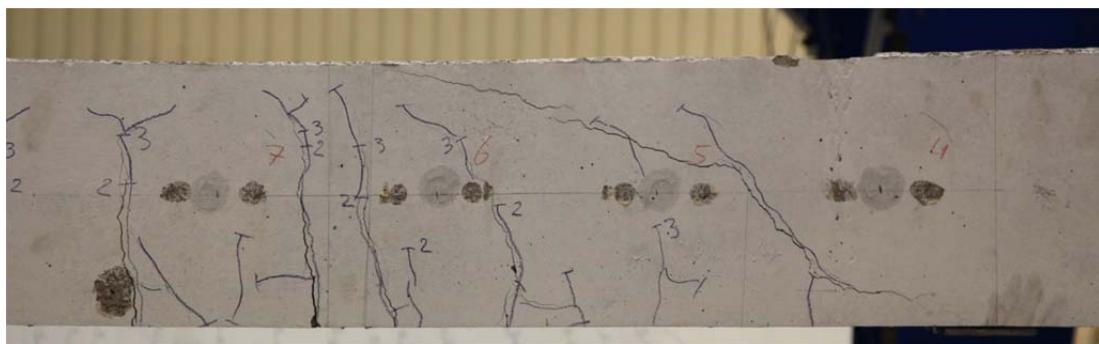
Fig. 5.30.2. Crack pattern after failure south side
