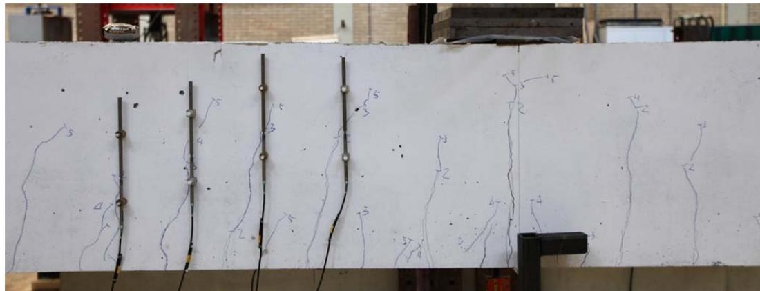
Fig. 5.43.1. Crack pattern after failure north side
