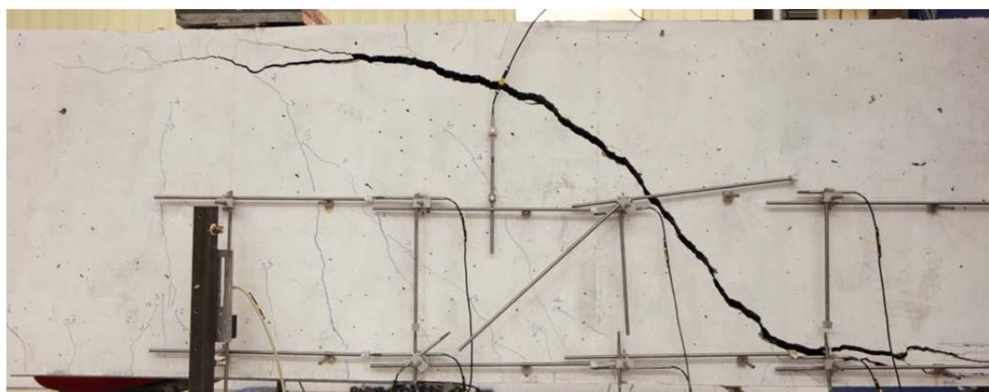
Fig. 5.87.2. Crack pattern after failure and LVDT layout at south side of beam
