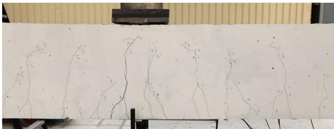
Fig. 5.50.2. Crack pattern after failure south side
