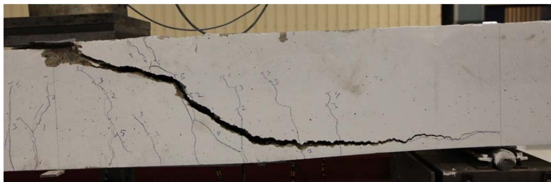
Fig. 5.61.2. Crack pattern after failure south side
