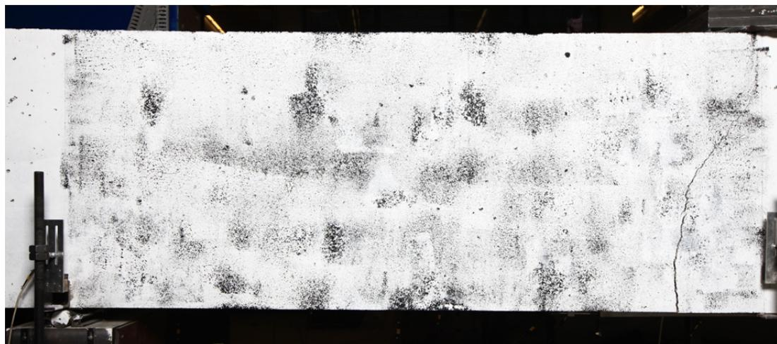
Fig. 5.83.1. Crack pattern after failure north side
