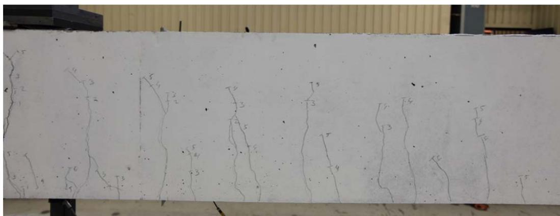
Fig. 5.40.2. Crack pattern after failure south side
