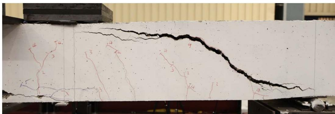
Fig. 5.60.2. Crack pattern after failure south side
