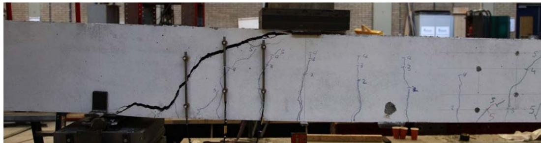
Fig. 5.37.1. Crack pattern after failure north side
