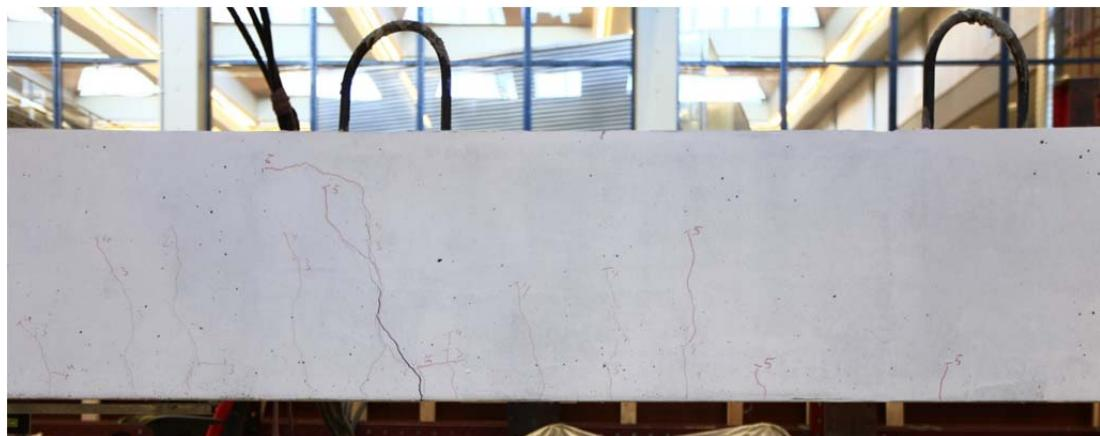
Fig. 5.76.1. Crack pattern after failure front side
