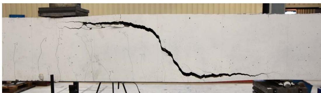
Fig. 5.49.2. Crack pattern after failure south side
