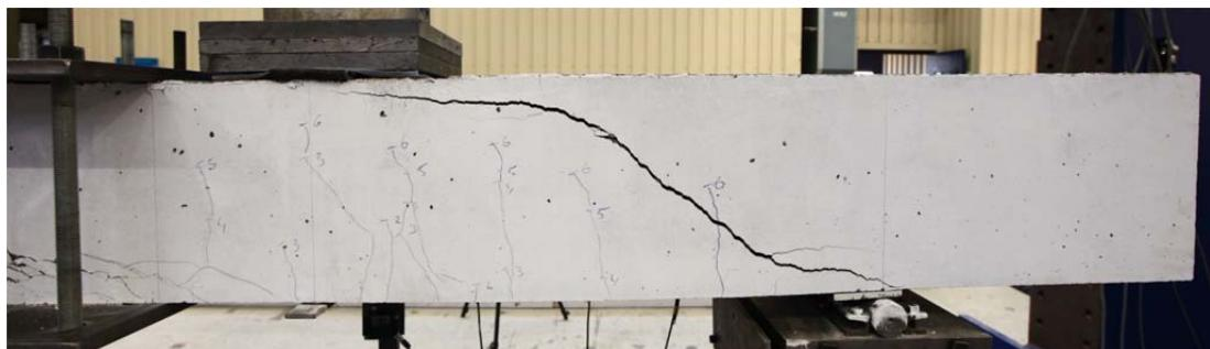
Fig. 5.9.2. Crack pattern after failure south side
