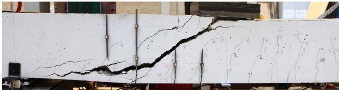
Fig. 5.55.1. Crack pattern after failure north side
