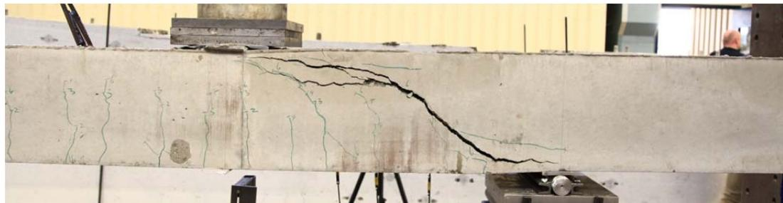
Fig. 5.15.2. Crack pattern after failure south side
