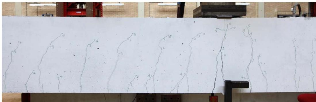
Fig. 5.40.1. Crack pattern after failure north side
