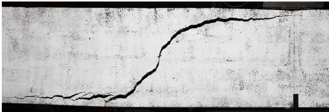
Fig. 5.98.1. Crack pattern after failure north side
