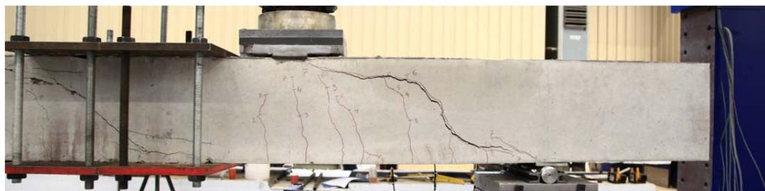
Fig. 5.16.2. Crack pattern after failure south side
