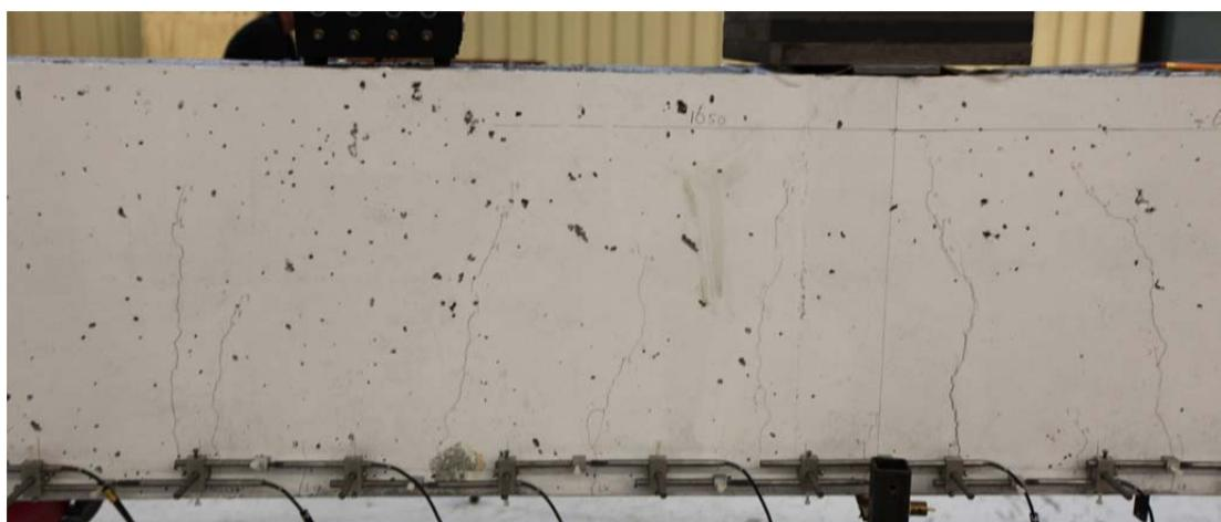
Fig. 5.82.2. Crack pattern after failure south side
