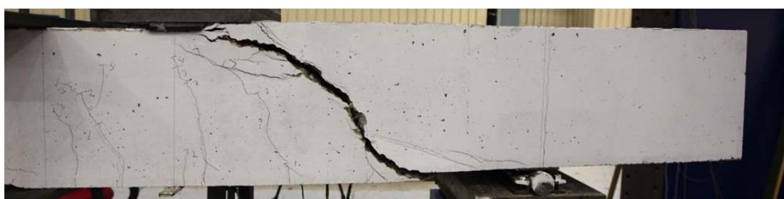
Fig. 5.65.2. Crack pattern after failure south side
