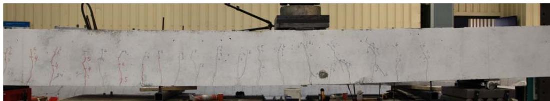
Fig. 5.20.2. Crack pattern after failure south side
