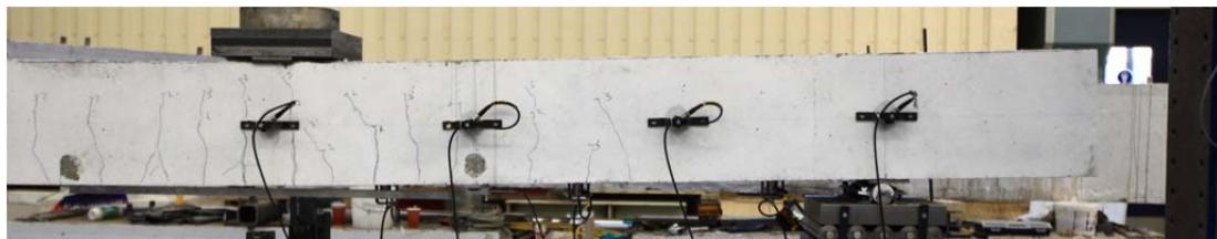
Fig. 5.38.3. Sensors used for Acoustic Emission measurements
