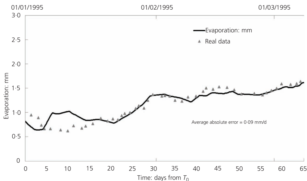
Figure 9. Results of numerical simulations and experimental data for the total daily evaporation. Experimental data were adopted from Gonzalez-sosa et al. (1999)
